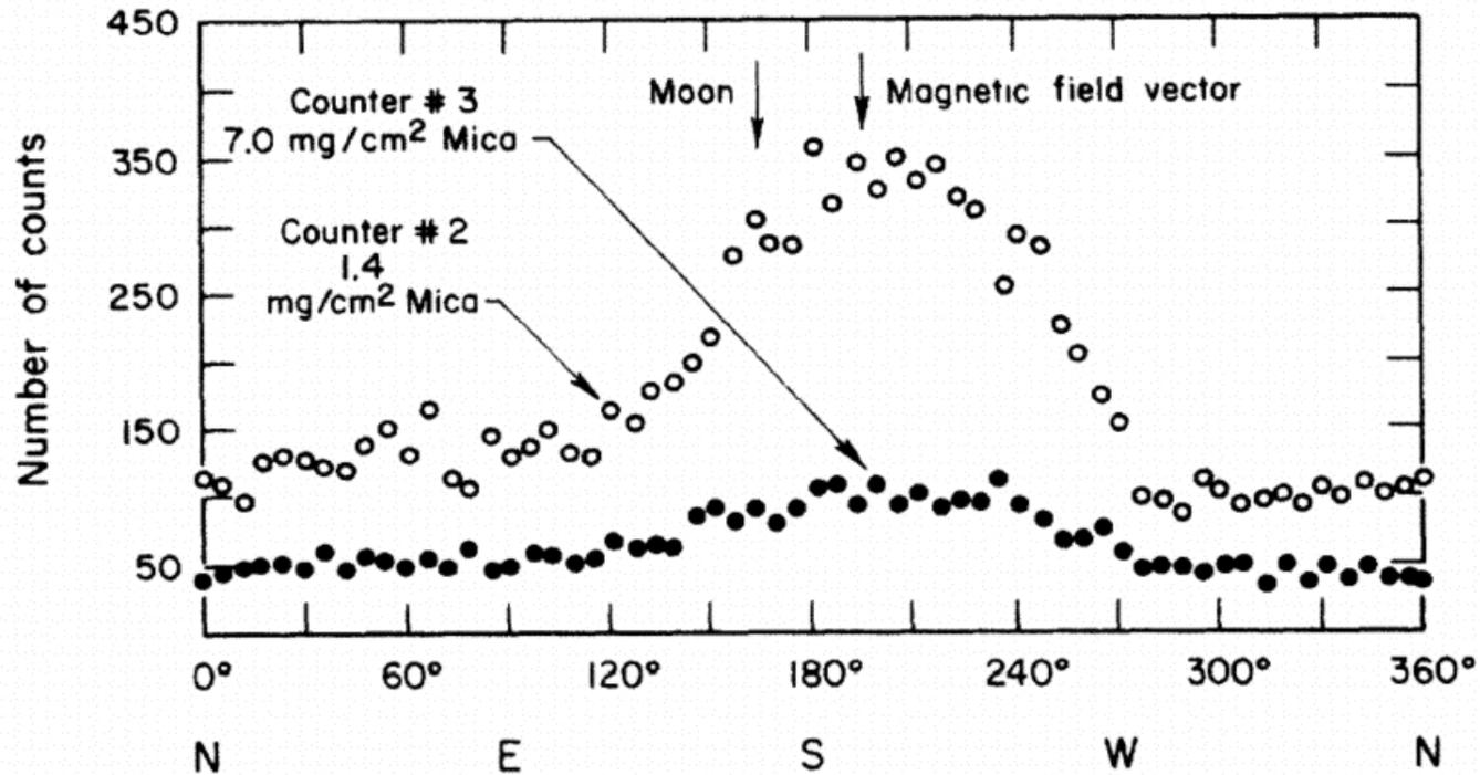
Number of counts versus azimuth angle. The numbers represent counts accumulated in 350 seconds in each 6-degree angular interval.
