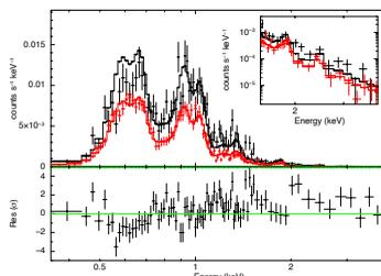
**Figure 3.** Source spectrum fit with the near background model. The red points and line are the near background data and model respectively. The black points are the source data and the black line is the fitted near background model with only the normalization free.
