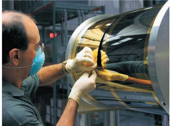
FIGURE 23: A prototype Con-X mirror segment being removed from a replication mandrel.
