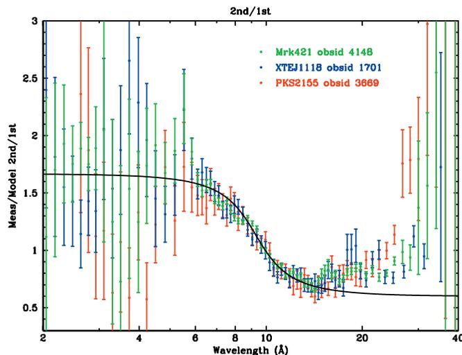
FIGURE 11: Comparison between measured and model ratios of 2nd/1st order LETG diffraction efficiencies (figure courtesy of Brad Wargelin).
