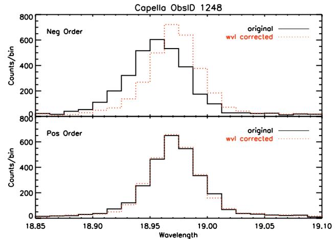
FIGURE 12: Capella line profiles for H-like O Ly $\alpha$  in negative and positive orders. Plotted in solid black are the standard-processed data, and in dotted red are the wavelength-corrected data. The improvement in the corrected data is more drastic for some lines than in others. In general, the wavelength-corrected data have smaller line widths, sharper peaks, and more accurate wavelength positions.
