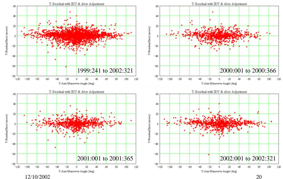
Y-Error Adjusted for IRU Calib 5.1, 5.2, 5.3, & Aberration vs Y-Axis Maneuver Angle
