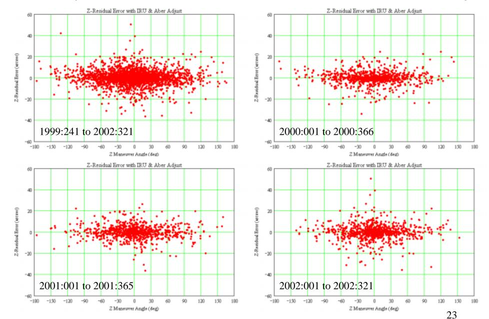
Z-Error Adjusted for IRU Calib 5.1, 5.2, 5.3, & Aberration vs Z-Axis Maneuver Angle
