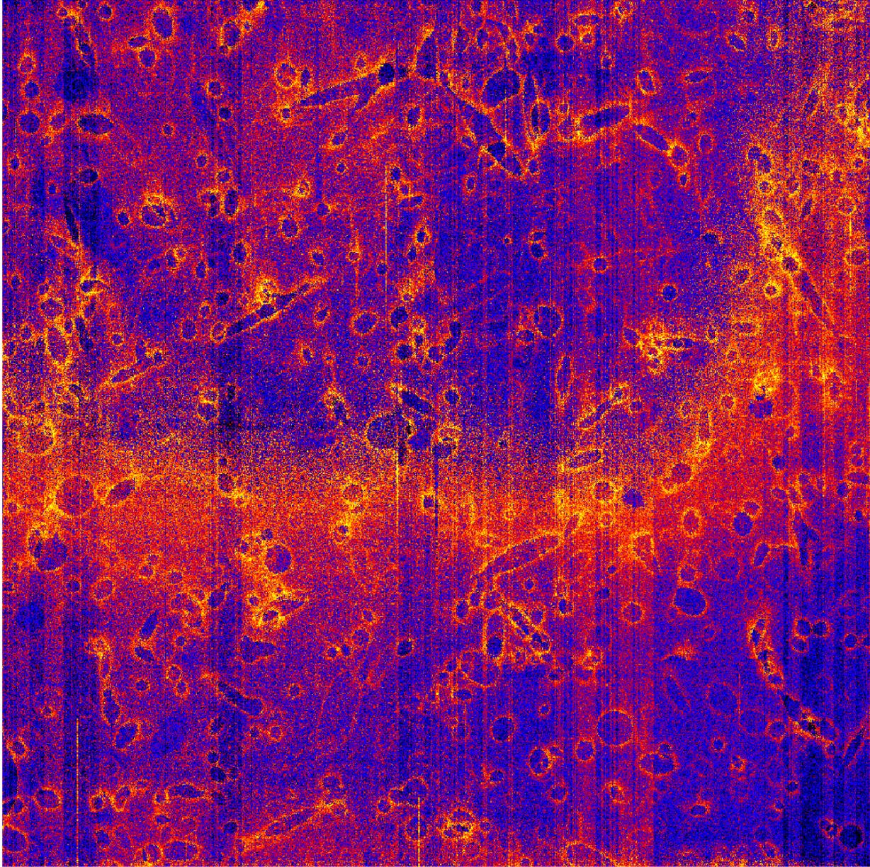
Figure 4. An unusual timed-exposure mode bias for a front-illuminated CCD (ACIS-I2). Large node-to-node offsets have been removed. An anomalous hook like feature is evident through the middle of the CCD from left to right and up the right-hand side.
