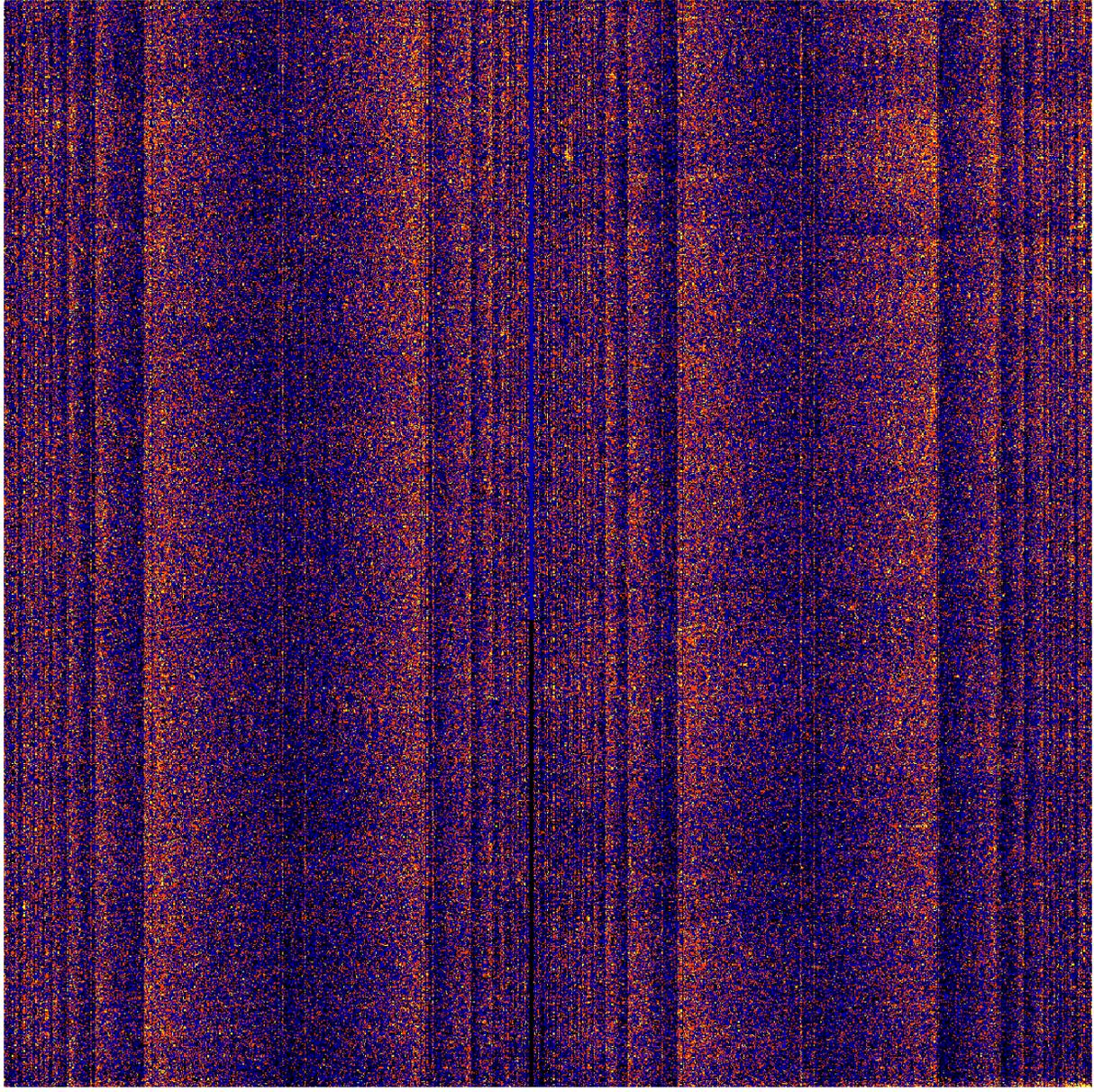
Figure 5. A nominal timed-exposure mode bias for a back-illuminated CCD (ACIS-S3). Large node-to-node offsets have been removed.
