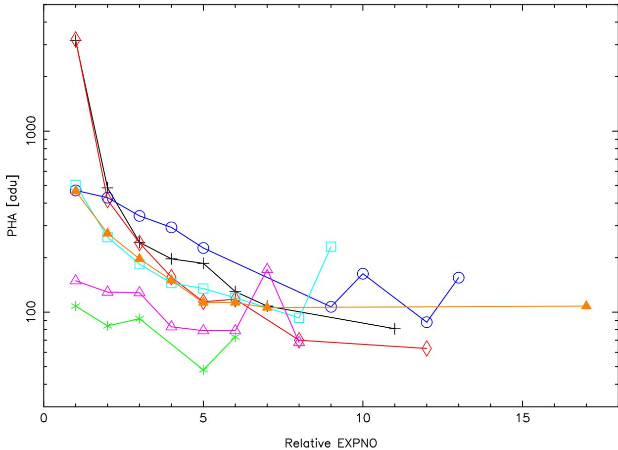
Figure 10. The pulse height (**PHA**) as a function of time (**EXPNO** or frame number) for a selected sample of afterglows. While the pulse height typically decreases from one event to the next, this trend is not universal. The pulse height can increase when the amount of charge “bottoms out” near the end of an afterglow. Also note that events do not have to occur in consecutive frames. There can be gaps.
