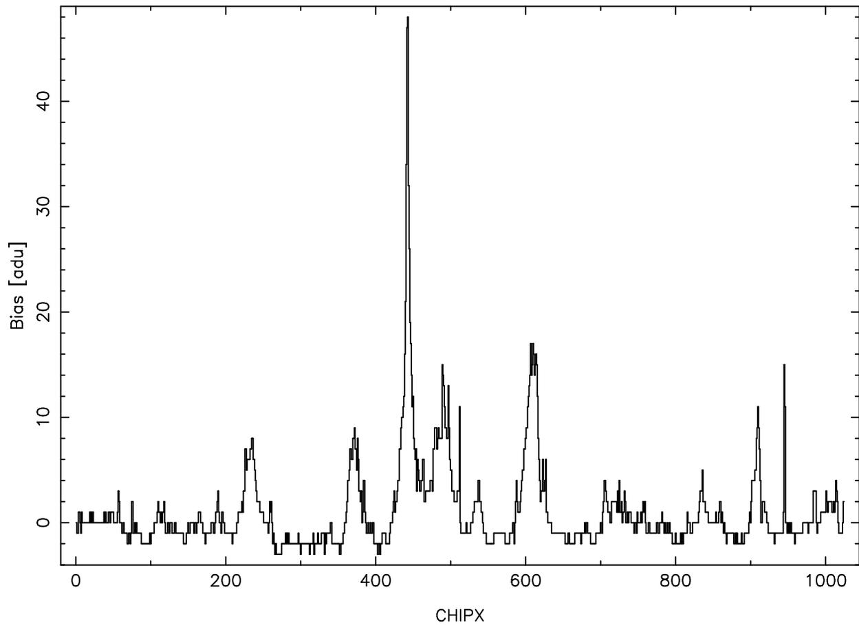
Figure 8. An “unusual” continuous-clocking mode bias for a front-illuminated CCD (ACIS-S2). Large node-to-node offsets have been removed. The anomalous peaks are caused charged particles.
