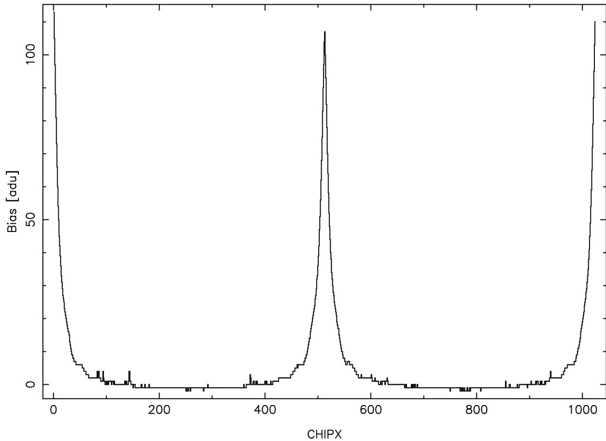
Figure 9. A nominal continuous-clocking mode bias for a back-illuminated CCD (ACIS-S3). Large node-to-node offsets have been removed. The peaks near the node boundaries at  $\text{CHIP} = 1, 512, 513,$  and  $1024$  are not unusual. They are due to a drop in the voltage.
