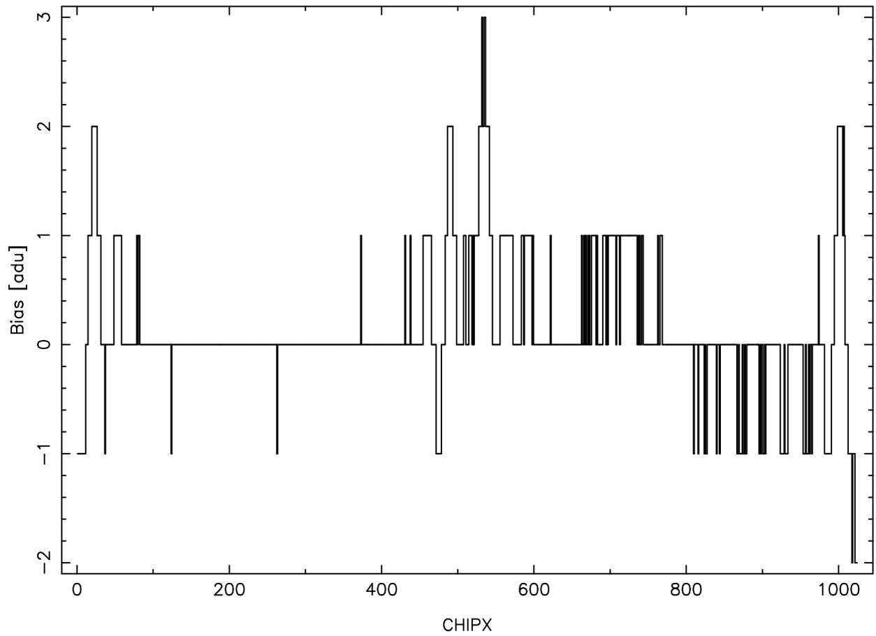
Figure 7. A nominal continuous-clocking mode bias for a front-illuminated CCD (ACIS-S2). Large node-to-node offsets have been removed.
