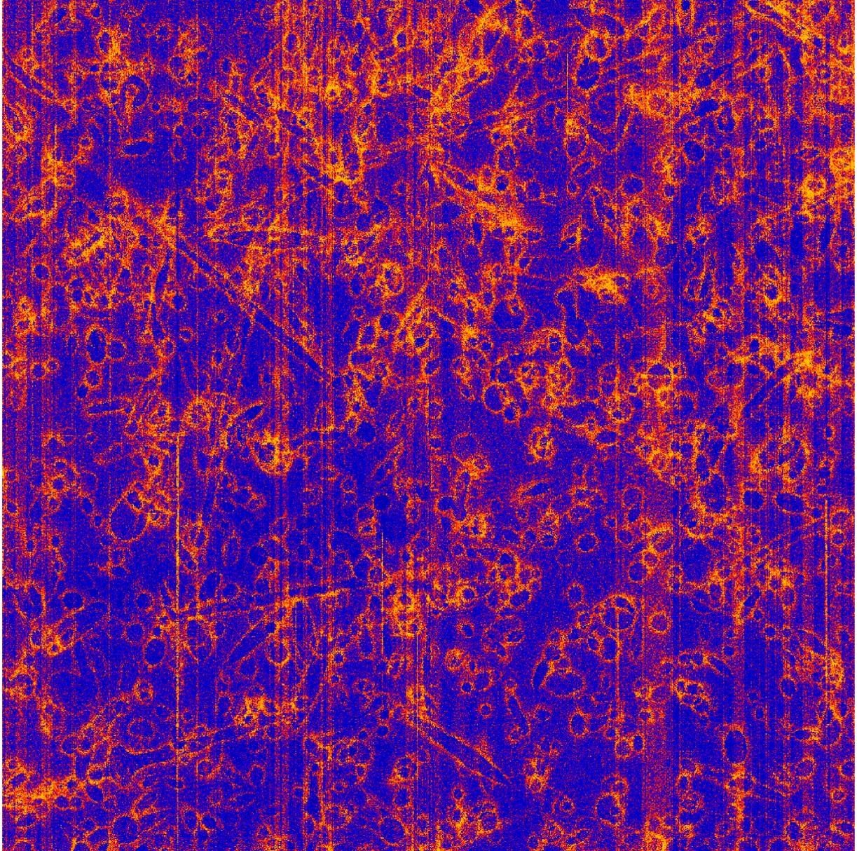
Figure 3. A nominal timed-exposure mode bias for a front-illuminated CCD (ACIS-I2). Large node-to-node offsets have been removed.
