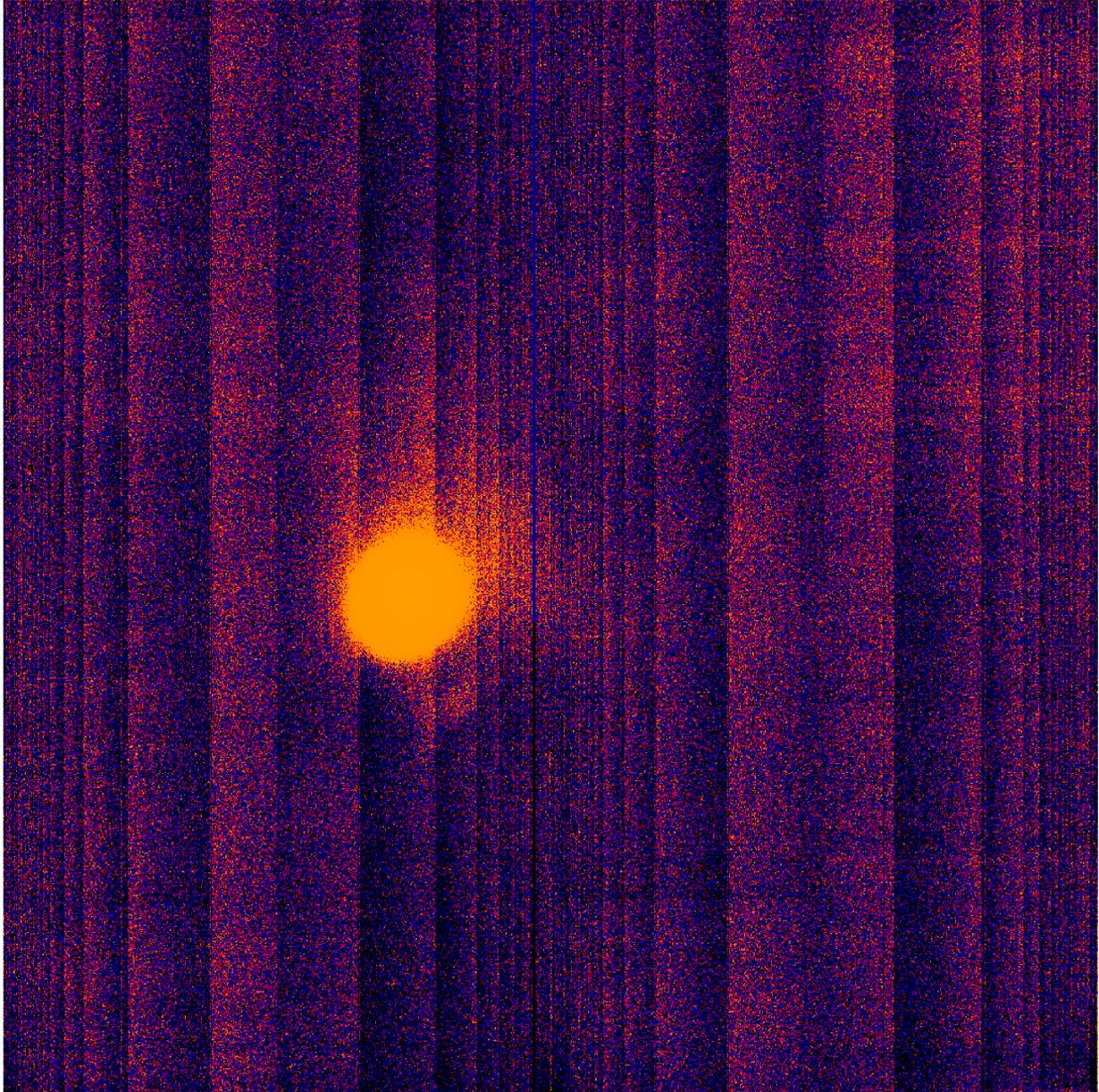
Figure 6. An unusual timed-exposure mode bias for a back-illuminated CCD (ACIS-S3). Large node-to-node offsets have been removed. The anomalous bright spot is source (Jupiter).
