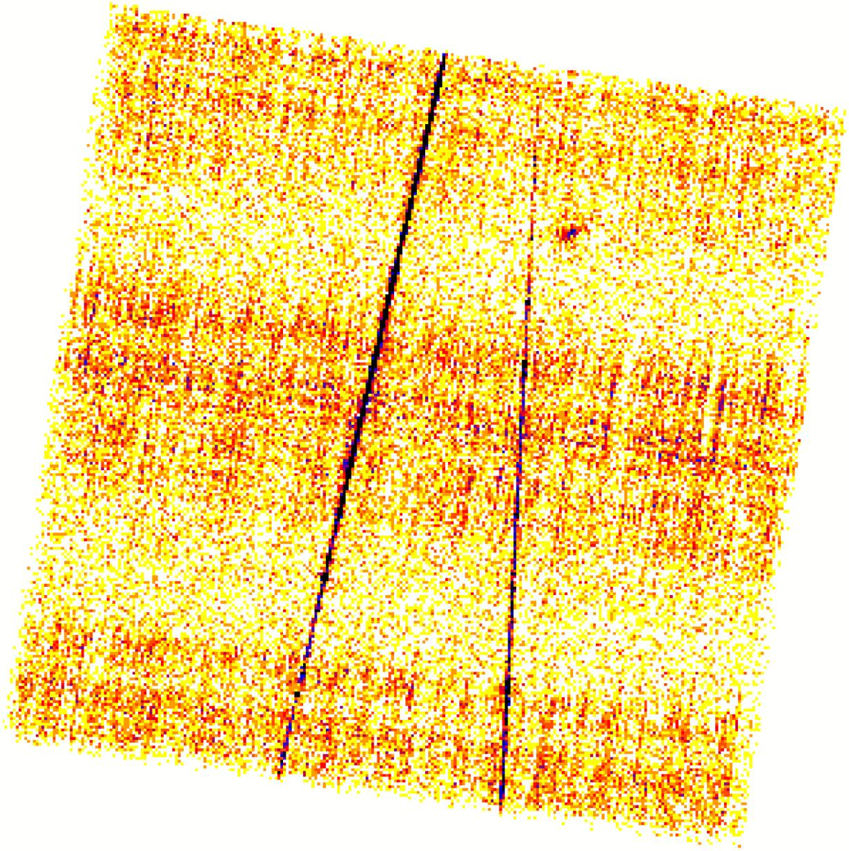
Figure 13. An image of the CCD ACIS-S4 before the horizontal streaks have been removed. The streaks are horizontal in chip, not sky, coordinates. The image also includes a source near the upper right-hand corner and portions of the HETG grating arms running through the middle of the CCD from the top to the bottom.
