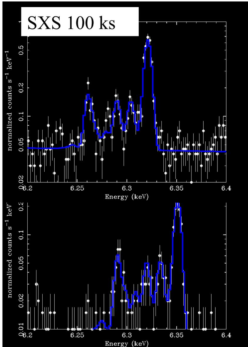
Using the SXS with an energy resolution better than 7eV, we could measure gas bulk motions in a fair number of X-ray bright clusters.
