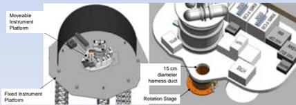
Four instrument are accommodated On moveable instrument platform, with grating CCD fixed on fixed instrument platform
