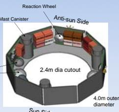
Note: Propulsion tank diameter and free path for x-rays through the middle determine the size of the spacecraft bus
