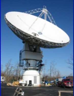
Figure 1: The Morehead State University 21-Meter Space Tracking Antenna (STA).
