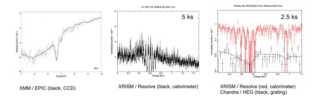
Map for the first time Fe L and Fe K simultaneously at high resolution!
