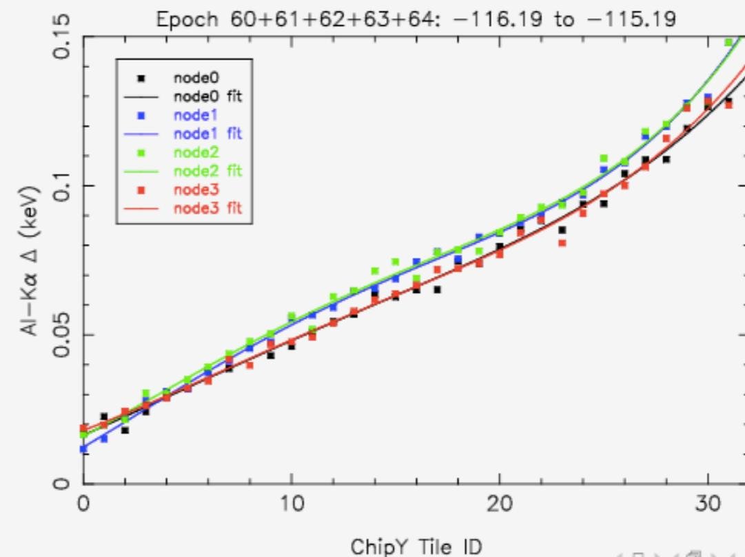
In the process of fitting ECS data taken over the course of mission with the goal of generating a set of time- and temperature-dependent scatter matrices.
