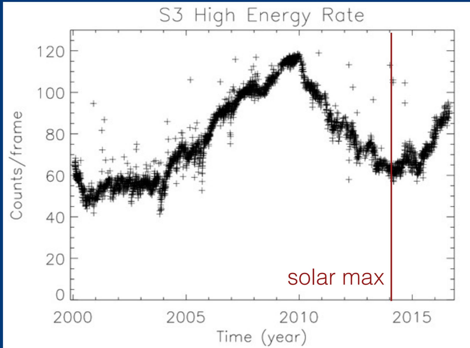
A new set of ACIS blank sky background files are being compiled. Now that data has been accumulated for more than a full solar cycle, studies can be carried-out to determine if there are any significant changes in the charge particle-induced detector background between cycles.
