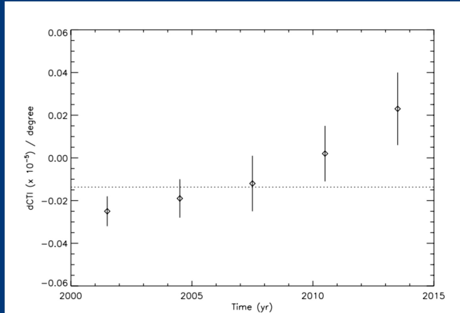
Up till now, a constant  $d(\text{CTI})/dT$  has been applied to ACIS data (the horizontal line). We are in the process of adjusting the CALDB so that the appropriate  $d(\text{CTI})/dT$  value, given the date of the observation, will be applied.
