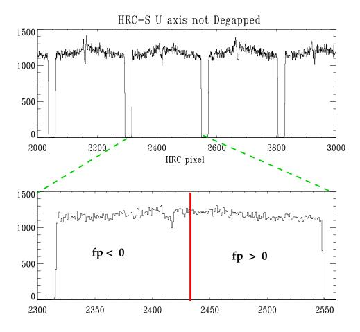
Fig. 4.— For projection of flat field we look at region between gaps. Each is broken into fine position > and < 0. The derivative of the fit to the distribution gives the function that corrects the non-linearity
