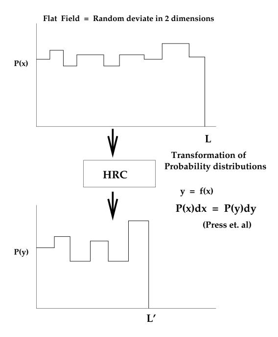
Fig. 5.— Proof of statement for previous figure can be derived by considering transformation of probability distributions. Input flat field is a random uniform deviate in two dimensions. HRC non-linearity transforms the simple input probability distribution
