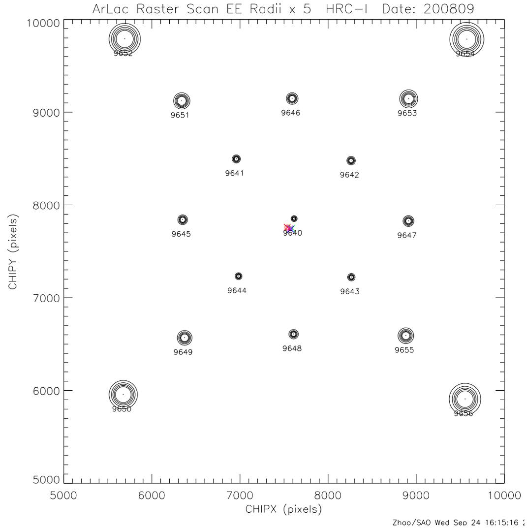
Figure 3: HRC-I raster scan of Ar Lac with 1ks exposure time for each point, except the center point which is 3ks (Date: 2008-09-07). Circles around each observation point are the 50%, 60%, 70%, 80%, 90% encircled energy circles  $\times 5$ .
