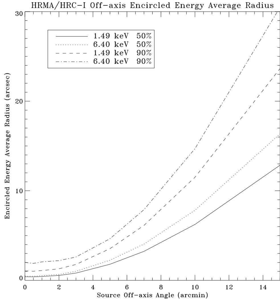
Figure 17: The HRMA/HRC-I Encircled Energy as a function of off-axis angle (POG.11: Figure 4.12). It shows that the current small separation ( $< 15''$ ) between the Optical Axis and the Aimpoint does not degrade the onaxis target PSF on the HRC.
