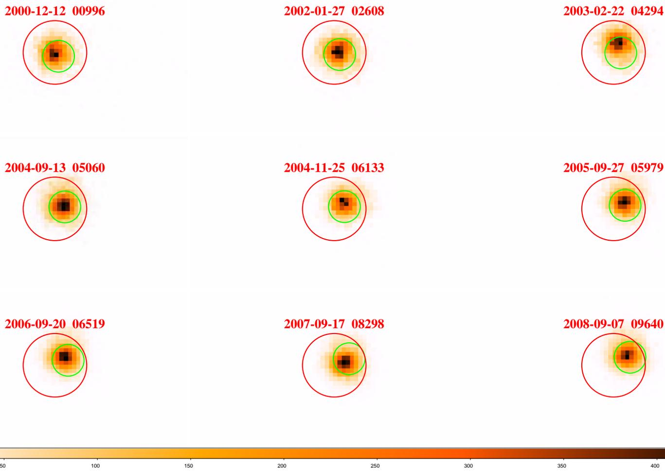
Figure 23: Chandra On-axis Point source (ArLac) HRC-I images in the past decade. The red circle ( $1''$  radius) is centered at its J2000 coordinate ( $RA_{\text{targ}}, Dec_{\text{targ}}$ ). The green circles ( $0.5''$  radius) are centered at the predicted positions at different observing times, based on its proper motion:  $\delta RA = -0.05248''/yr$ ,  $\delta Dec = 0.04788''/yr$ . The image quality stays the same, and the pointing is very accurate.
