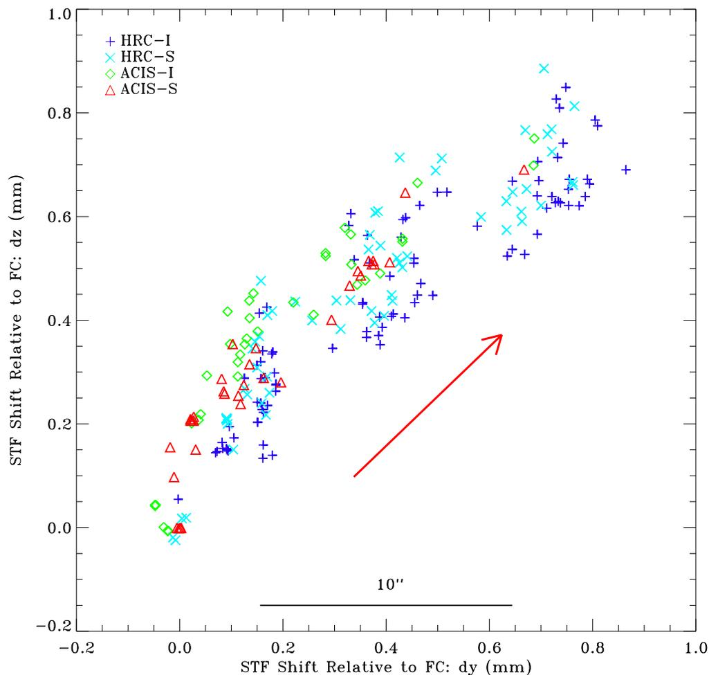
Figure 11: STF drifted about 1.2mm (24'') in +SIM-Y and +SIM-Z direction since launch.
