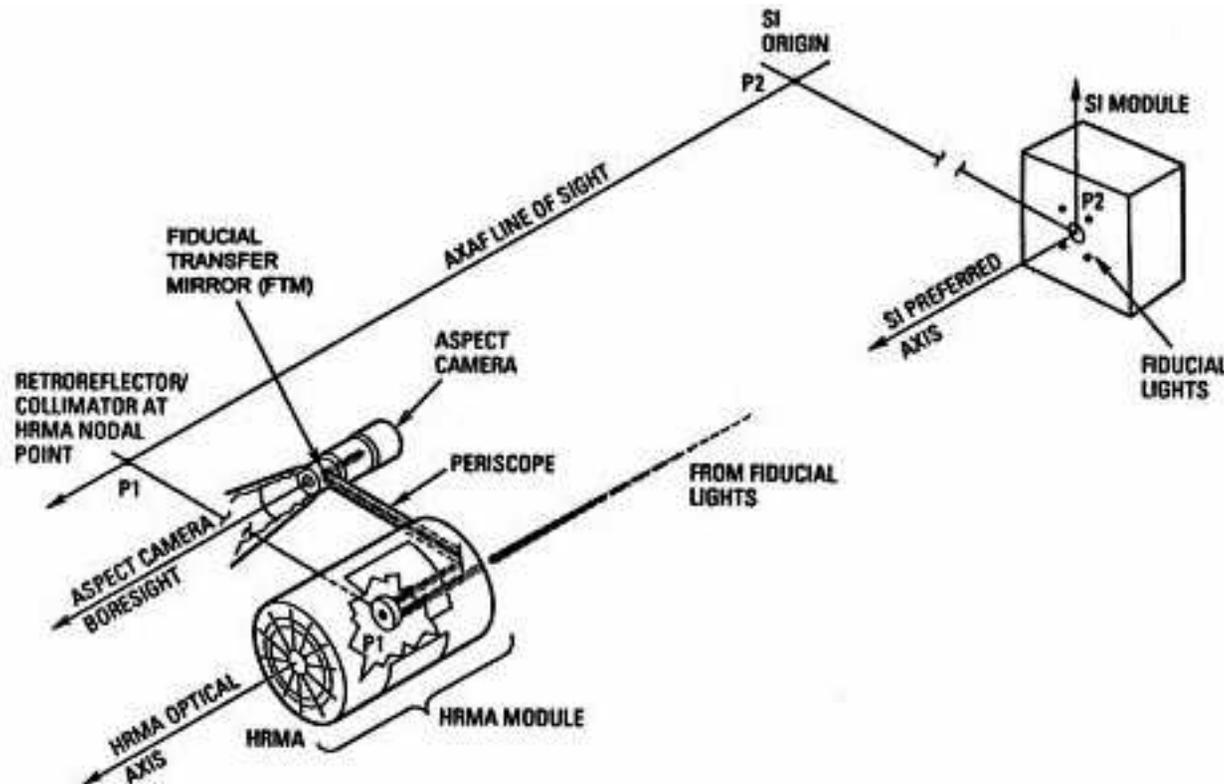
Figure 1: Chandra Pointing and Fiducial Transfer System. (POG.11: Figure 5.3.)
