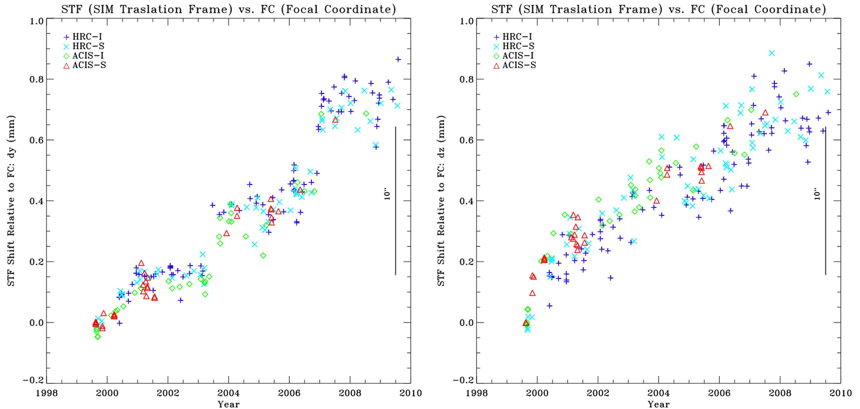
Figure 9: STF dy drifted about 0.9mm (18'') since launch. Figure 10: STF dz drifted about 0.9mm (18'') since launch.
