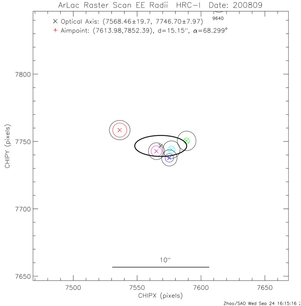
Figure 5: Optical Axis and Aimpoint position on HRC-I, based on raster scan observation of Ar Lac made on 2005-09-17. The Optical Axis is the weighted average of five EE (50% – 90%) measurements, at the center of the error ellipse.
