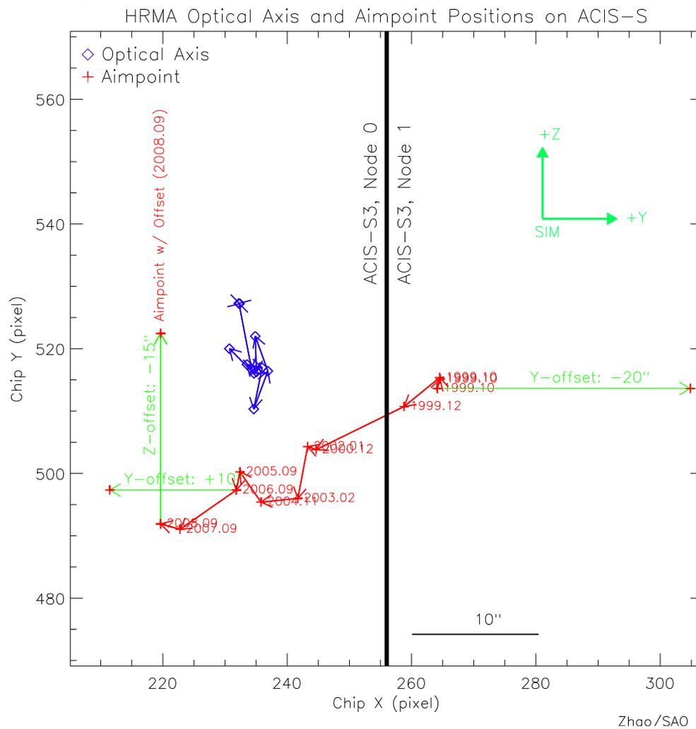
Figure 21: Chandra Optical Axis and Aimpoint positions on ACIS-S, transformed from the HRC-I measurements. Because of the aimpoint drift, the default target pointing offset for ACIS-S observations has been implemented three times to avoid the dither pattern falls on the node boundary: 1) Y-offset= $-20''$  in Oct. 1999; 2) Y-offset= $+10''$  in Sept. 2005; and 3) Z-offset= $-15''$  in Jan. 2007. The last one is to put the target pointing closer to the Optical Axis.
