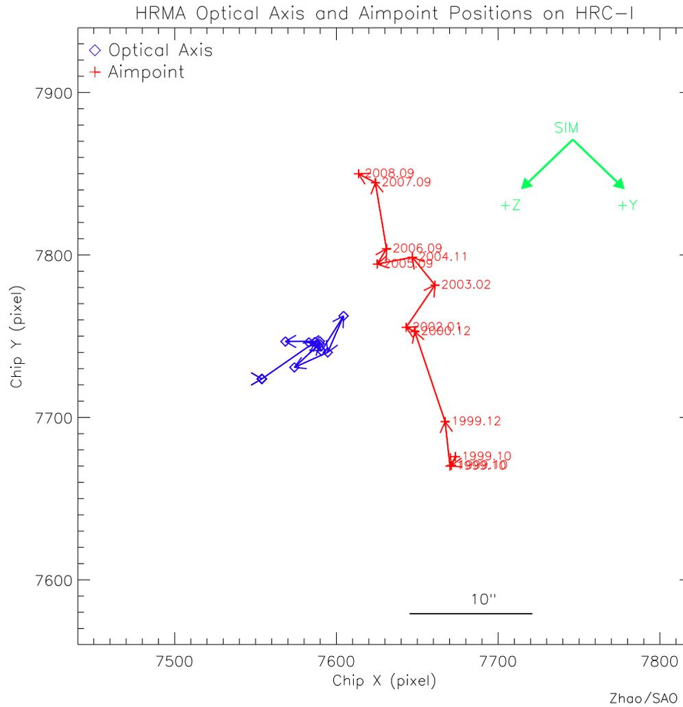
Figure 8: Optical Axis and Aimpoint positions from all the HRC-I measurements on CHIP coordinates. The Aimpoint has drifted by more than 24'' in the -Y and -Z direction of the SIM coordinates. But the two points were never more than 16'' apart.
