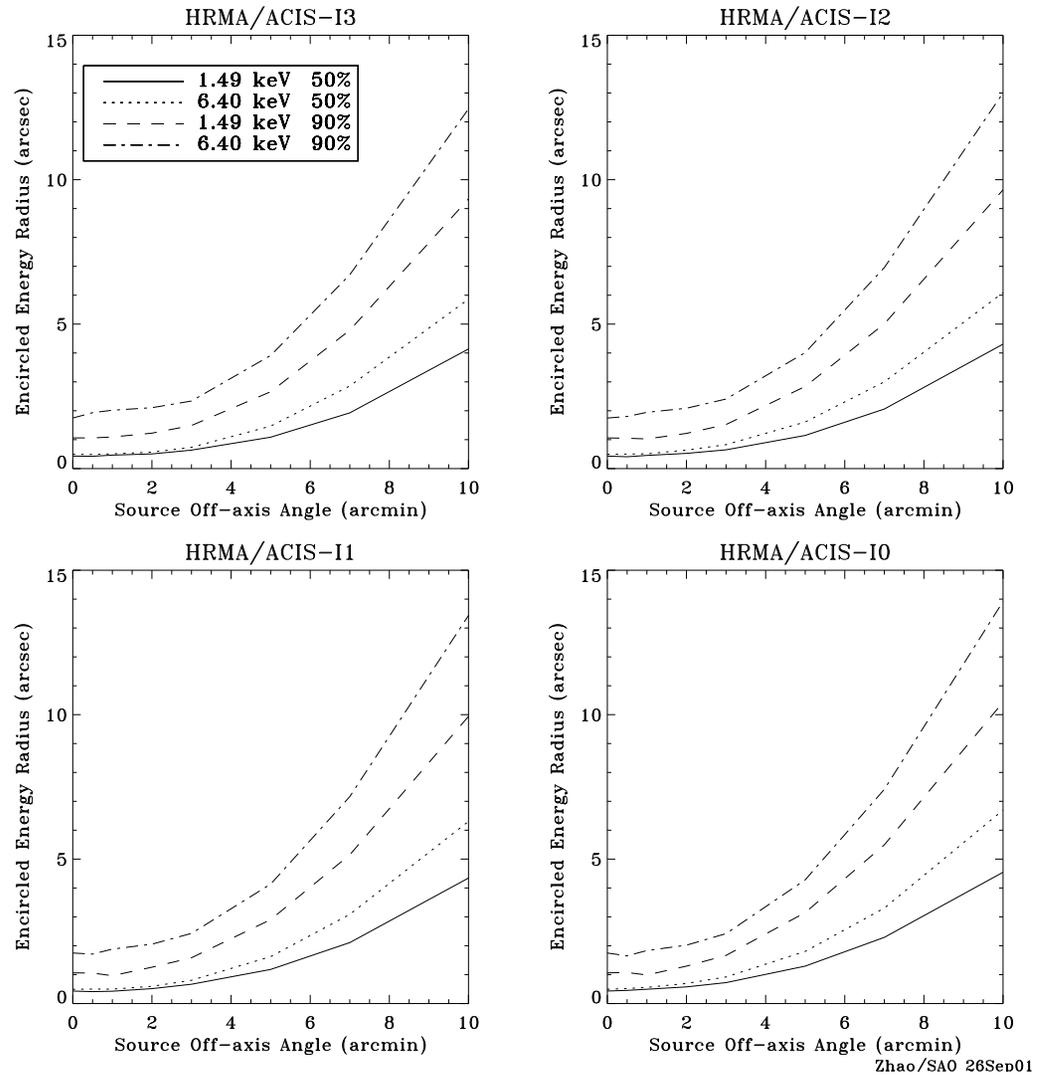
Figure 18: The HRMA/ACIS-I Encircled Energy as a function of off-axis angle (POG.11: Figure 4.13). It shows that the current small separation ( $< 15''$ ) between the Optical Axis and the Aimpoint does not degrade the onaxis target PSF on the ACIS.
