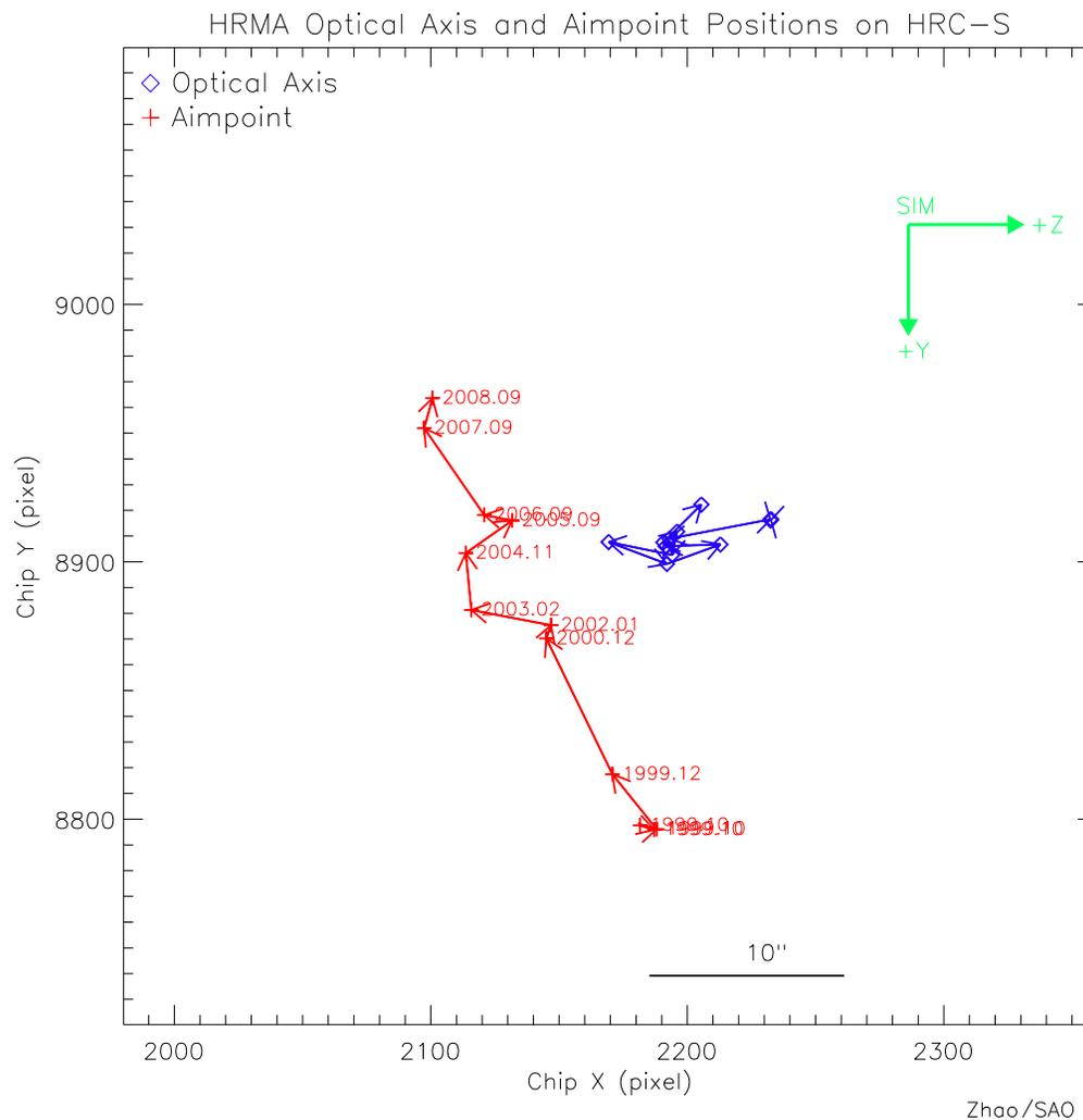
Figure 16: Chandra Optical Axis and Aimpoint positions on HRC-S, transformed from the HRC-I measurements.
