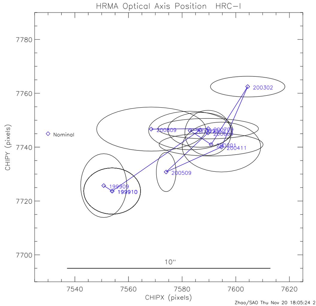
Figure 6: Optical Axis positions from all the HRC-I measurements on CHIP coordinates. The drift of the Optical Axis is more like a random walk within 10".
