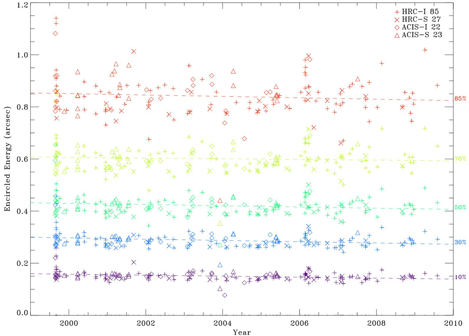
Figure 27: Chandra On-axis Encircled Energy of point sources on all four detectors. The EE did not change since launch. i.e. the Chandra image quality (PSF) stays the same with superb spacial resolution.
