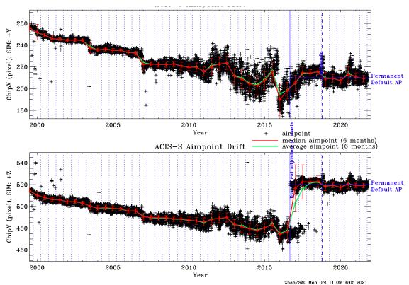
Figure 16: Aimpoint position as a function of time on ACIS-S since launch. Solid red (green) lines show the median (average) aimpoint drift in 6 month bins, separated by vertical dotted blue lines. The vertical solid blue line indicates the start of the dynamical aimpoint adjustment.
