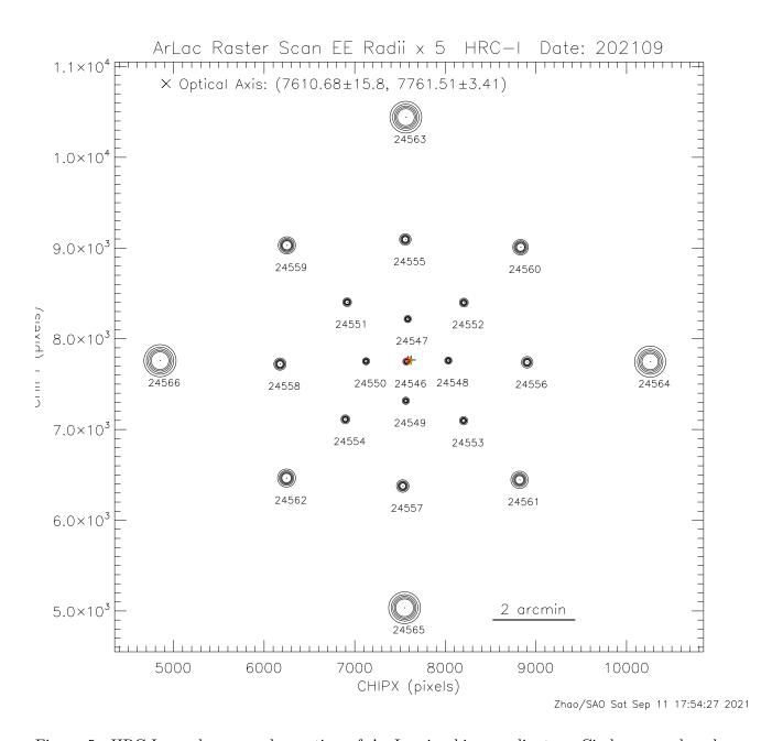
Figure 5: HRC-I annular scan observation of Ar Lac in chip coordinates. Circles around each observation point have the 50%-90% encircled energy radii  $\times$  5. The data are fit to a 2-D quadratic function to find the optical axis. Data taken in September 2021. The numbers under the circles are the OBSIDs of the observations.
