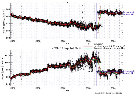
Figure 14: Aimpoint position as a function of time on ACIS-I since launch. Solid red (green) lines show the median (average) aimpoint drift in 6 month bins, separated by vertical dotted blue lines. The vertical solid blue line indicates the start of the dynamical aimpoint adjustment.
