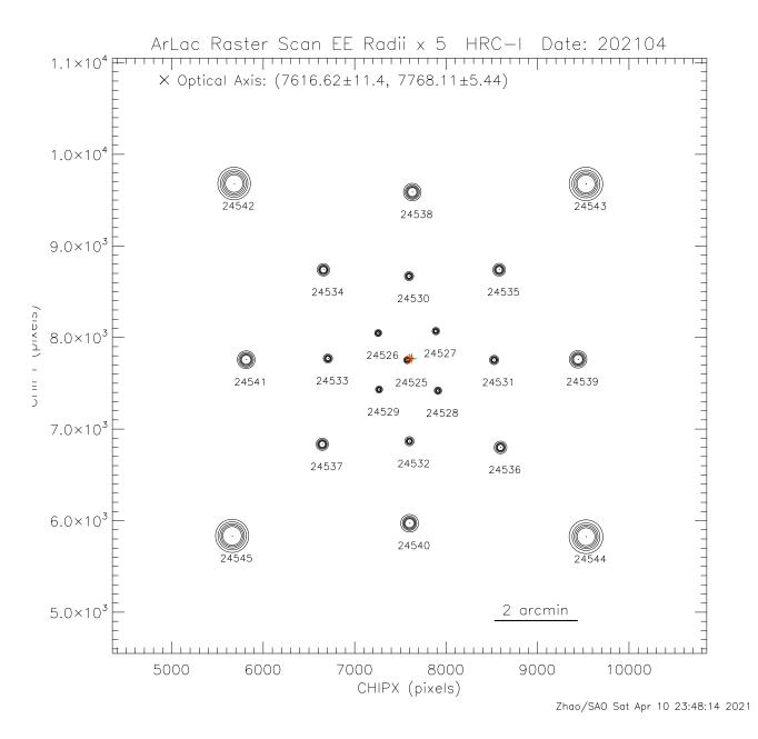
Figure 4: HRC-I annular scan observation of Ar Lac in chip coordinates. Circles around each observation point have the 50%-90% encircled energy radii  $\times$  5. The data are fit to a 2-D quadratic function to find the optical axis. Data taken in April 2021. The numbers under the circles are the OBSIDs of the observations.
