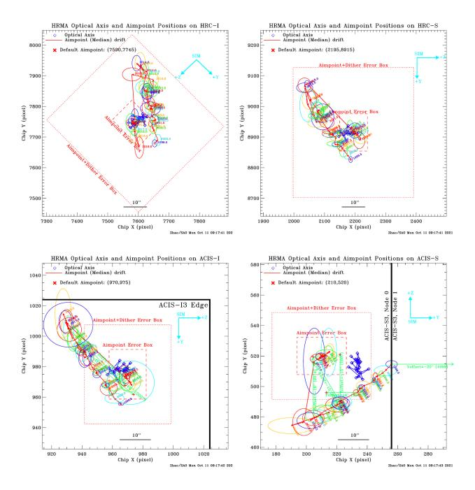
Figure 22: Same as Figures 18 – 21, the optical axis (blue) and median aimpoint (red) drifts on HRC-I (upper-left), HRC-S (upper-right), ACIS-I (lower-left) and ACIS-S (lower-right), with the colored ovals indicating the 1- $\sigma$  error ellipse for data in a given half year bin.
