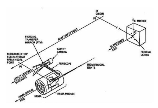
Figure 1: Chandra Pointing and Fiducial Transfer System. (POG: Figure 5.3.)
