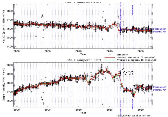
Figure 10: Aimpoint position as a function of time on HRC-I since launch. Solid red (green) lines show the median (average) aimpoint drift in 6 month bins, separated by vertical dotted blue lines. The vertical solid blue line indicates the start of the dynamical aimpoint adjustment.
