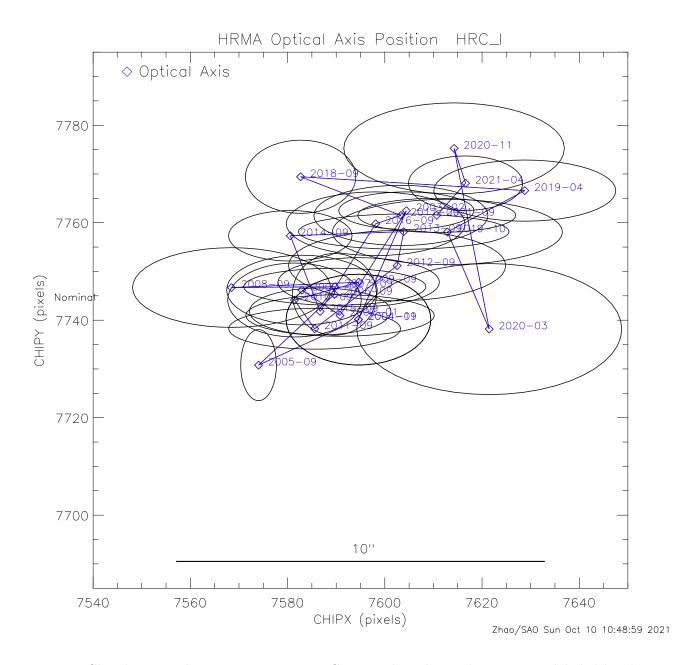
Figure 8: Chandra optical axis positions on HRC-I since launch. Each position is labeled by the year–month. The ellipse around each position is the  $1-\sigma$  measurement error ellipse for that given year. The drift of optical axis position is consistent with the measurement errors. The optical axis position is very stable and well within a 10'' region.
