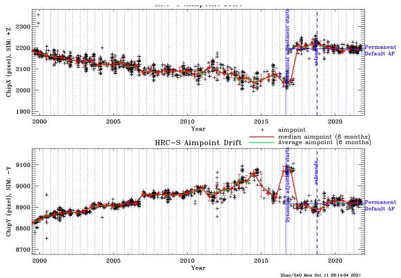
Figure 12: Aimpoint position as a function of time on HRC-S since launch. Solid red (green) lines show the median (average) aimpoint drift in 6 month bins, separated by vertical dotted blue lines. The vertical solid blue line indicates the start of the dynamical aimpoint adjustment.
