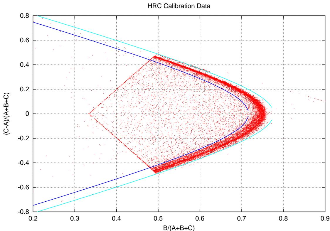
Figure 6: The same data as in Figure 5. Here the boundaries of the zone of acceptance are plotted. They are constructed from the best fit hyperbola to the good event locus offset by  $\pm 0.030$  in the  $f_b$  axis.
