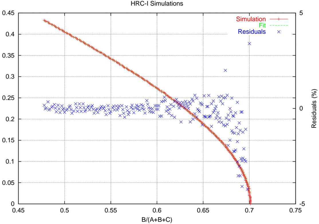
Figure 4: Fit of hyperbolic function to the simulated HRC. The best fit parameter values are  $a=0.3353(0.3720)$ ,  $b=0.3263(0.3454)$ ,  $h=1.0364(1.0738)$ . The two curves are virtually identical. Also shown are the residuals between the simulated data and the best fit hyperbola.
