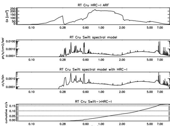
Predicted response in the HRC-I based on the best-fit Swift spectrum. From top to bottom, the panels are: The HRC-I effective area; the best-fit spectral model; the predicted counts spectrum in the HRC-I; and the cumulative counts spectrum. Notice that the nominal spectral model could be supplemented by a soft component that would be observable only with the HRC-I, to account for the difference in the predicted and observed rates.
