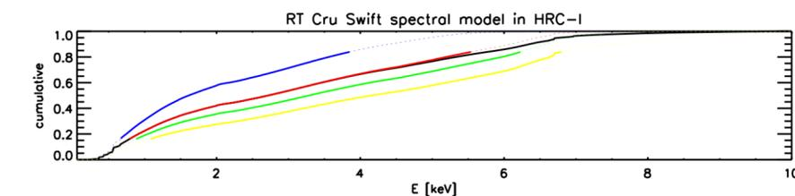
Cumulative predicted HRC-I count rates due to Chandra Mirror shells 1 (blue), 3 (red), 4 (green), and 6 (yellow). The solid segments denote the central 68% of the spectra. High energy photons are predominantly reflected by Shells 3, 4, and 6.
