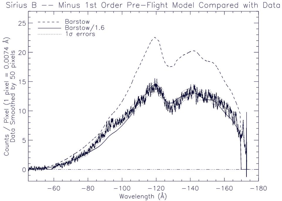
**Figure 4.** Comparison of the pre-flight model-predicted spectrum for Sirius B with the LETGS observed spectrum indicate that the pre-flight low energy HRC-S QE is overestimated by an average factor of about 1.6. Dashed line is the model, solid line is the model/1.6, and dotted lines are the  $1\sigma$  statistical errors on the data. Positive and negative orders plotted separately.
