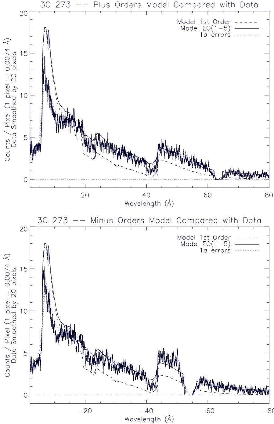
**Figure 9.** Comparison of the 1st order model-predicted spectrum (dashed curve) and the  $\Sigma O(1-5)$  model-predicted spectrum (solid curve) for 3C 273 with the LETGS observed spectrum. The summed orders model shows good agreement with the observed spectrum over the energy range 0.2–0.8 keV, illustrating the significance of high order contributions. Positive and negative orders plotted separately.
