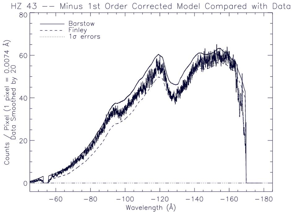
**Figure 8.** Comparison of two different model-predicted spectra for HZ 43 with the LETGS observed spectrum. Both models show good overall agreement with the data to  $\approx 10\%$ . Positive and negative orders plotted separately.
