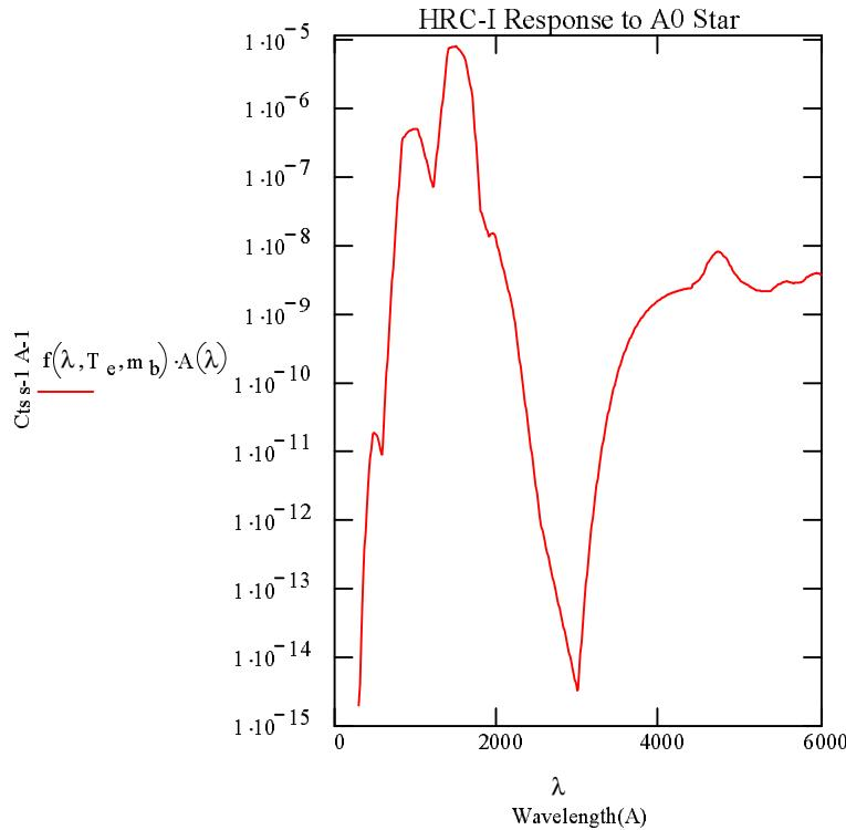
The estimated count rate for HRC-I in the band 300 - 6000 Å is the area under this curve:
