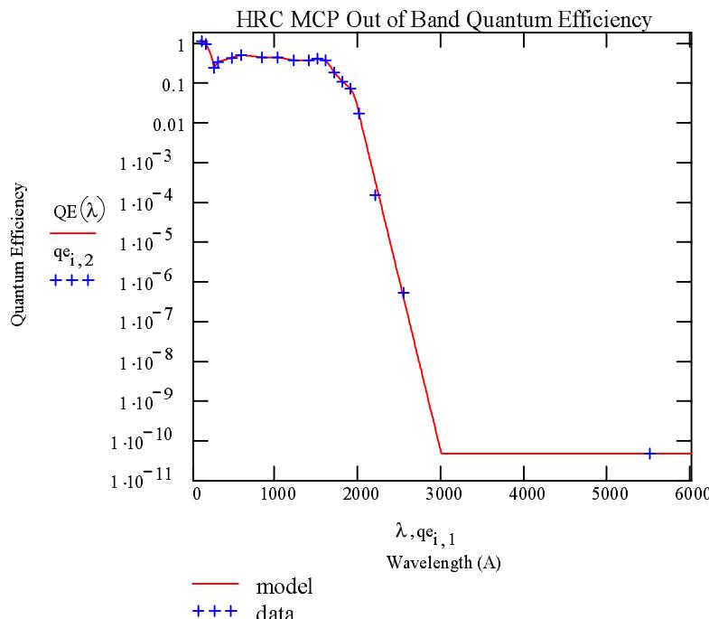
We will make a linear interpolation to define  $\mu$  for polyimide over the band 100-3000 A.
