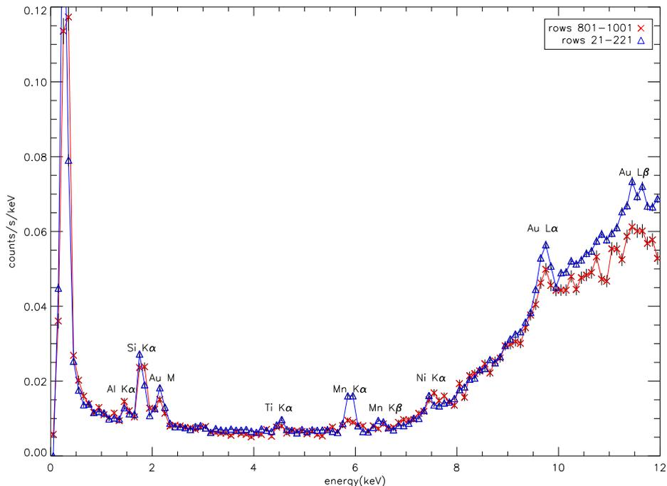
Figure 1: Composite Histogram Mode Background Spectra for the S3 chip. Energy is binned in units of 0.1 keV. Notable spectral features are labeled.
