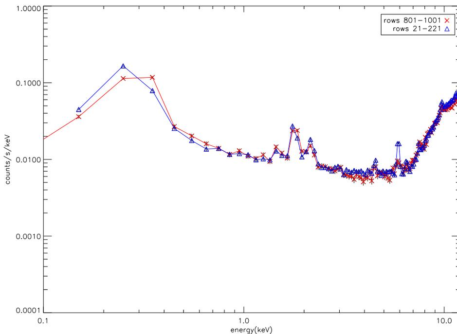
Figure 2: Composite Histogram Mode Background Spectra for the S3 chip. Energy is binned in units of 0.1 keV. X and Y axes are plotted logarithmically.
