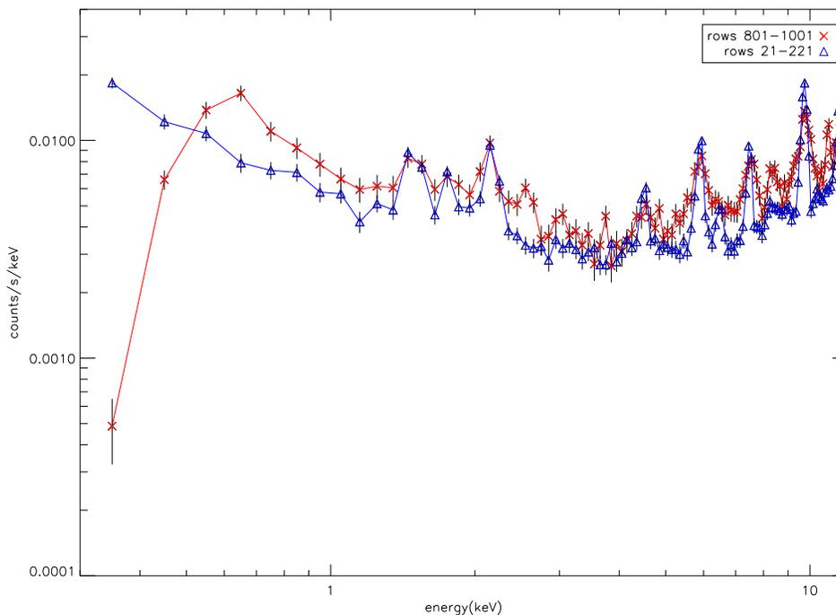
Figure 4: Composite Histogram Mode Background Spectra for the I3 chip. Energy is binned in units of 0.2 keV. X and Y axes are plotted logarithmically.
