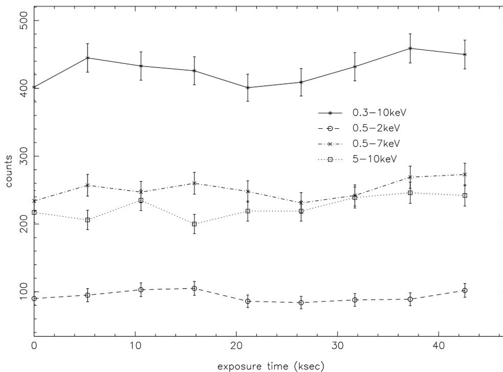
Figure 8: Counts per histogram file vs. elapsed time from beginning of exposure for the 0.3-10 keV, 5-10 keV, 0.5-2 keV, and 0.5-7 keV energy bands on I3 during obsid 27 (top). Each histogram file has an exposure time of 5.3 ksec.
