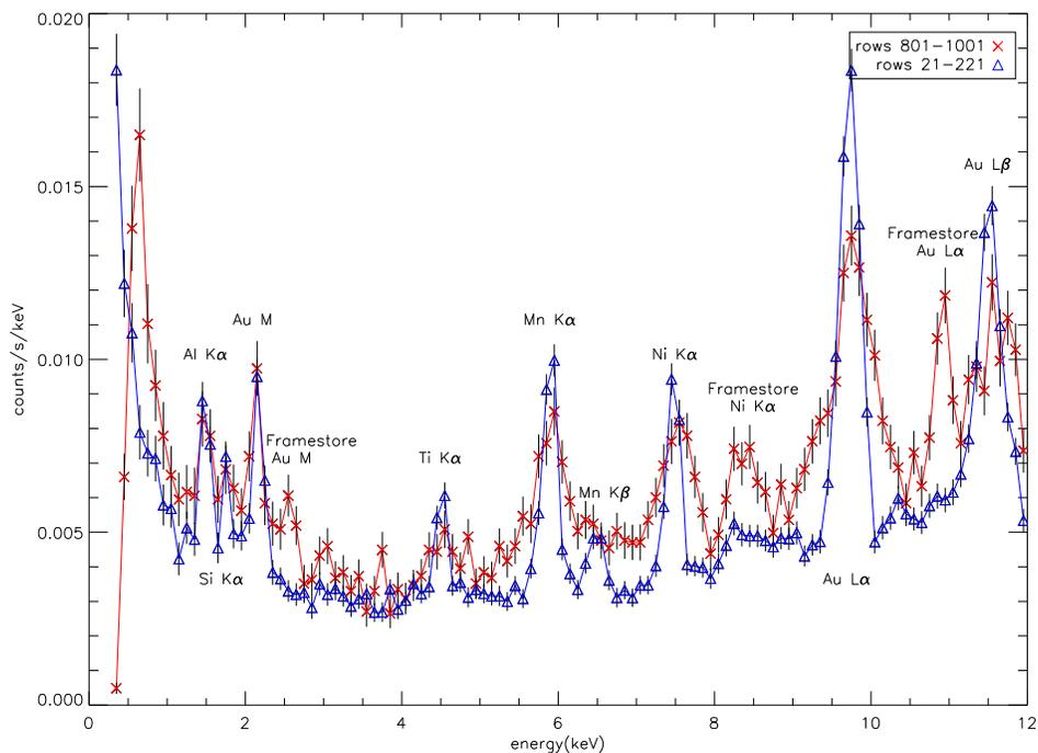
Figure 3: Composite Histogram Mode Background Spectra for the I3 chip. Energy is binned in units of 0.2 keV. Notable spectral features are labeled.
