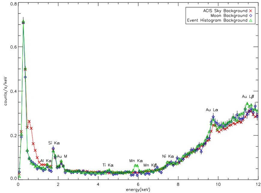
Figure 11: Overlay of ACIS sky background, moon background, and event histogram background for S3. Countrates in the histogram file background spectra have been corrected for the whole chip. All spectra are binned in units of 0.1 keV. Notable spectral features are labeled.
