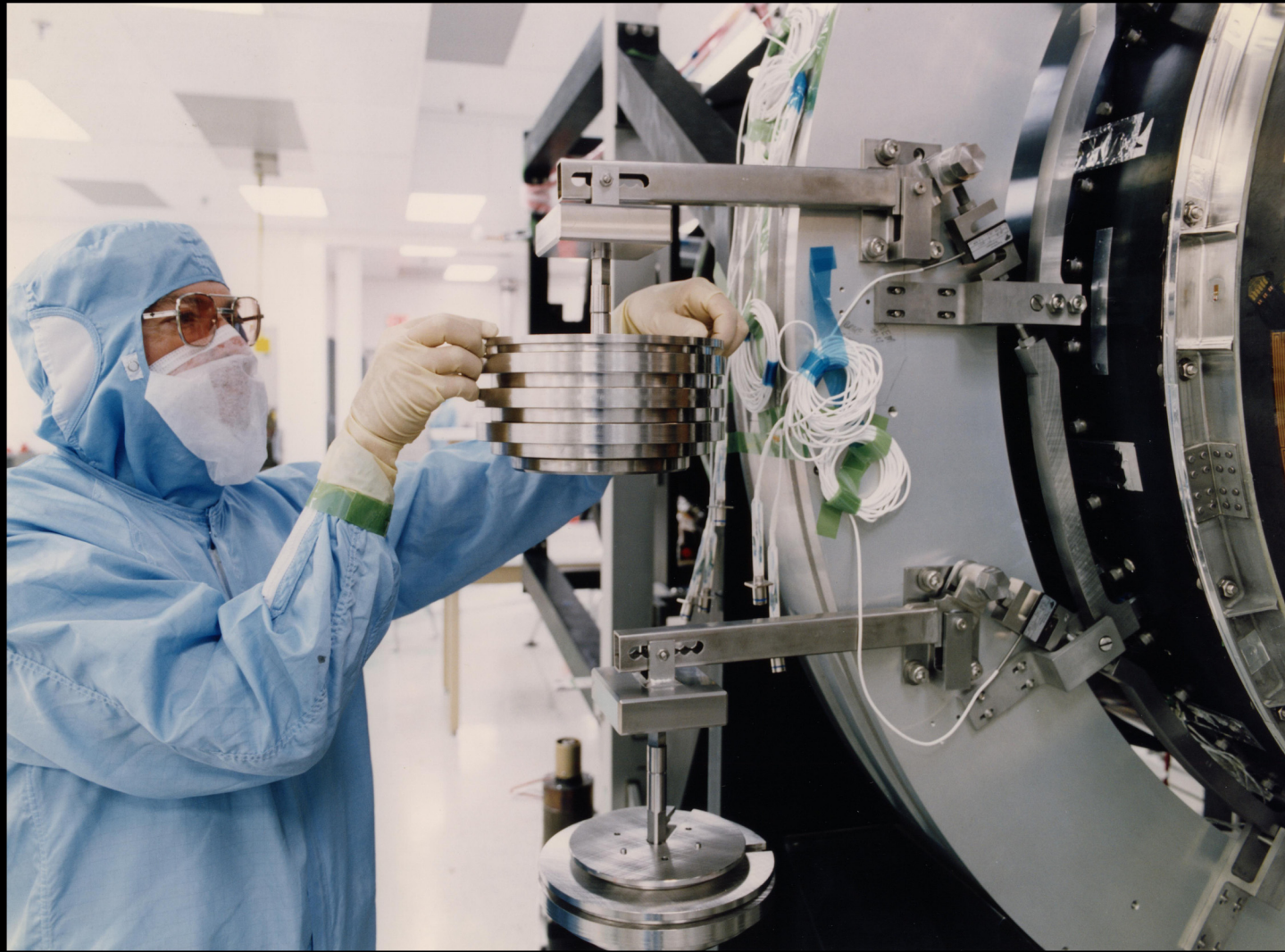
HRMA Offloaders being positioned prior to test
