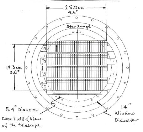
A Rows of 28 CCD's each ⇒ 112 CCD's total Fach CCD - 2400 × 600 13 × 13 × 13 × pixels Array 16,800 × 9,600 pixels ⇒ 161 Megapixels total
