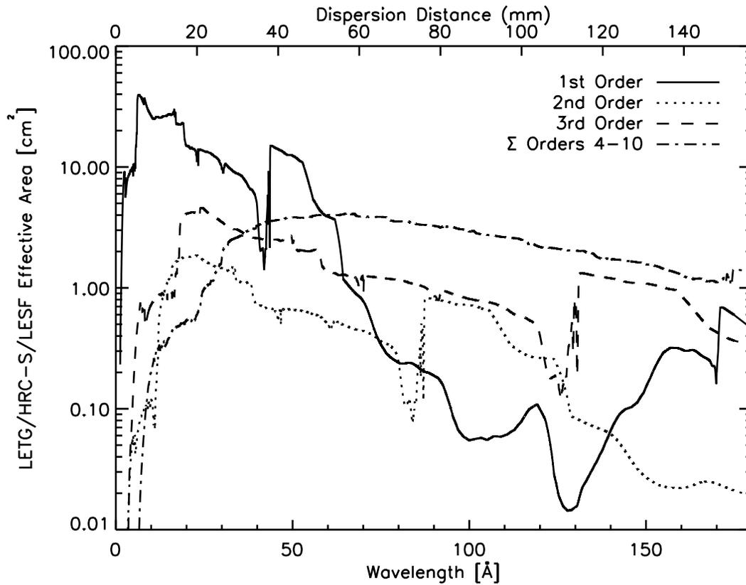
Figure 9.19: The combined HRMA/LETG/HRC-S/LESF effective areas for 1st and higher orders. Positive and negative orders are summed. Note that the wavelength axis begins at 10 Å.
