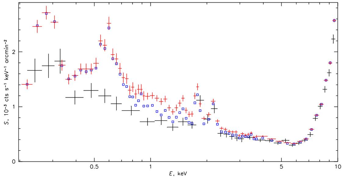
Figure 6.27: ACIS-S3 spectrum of the non-X-ray background (large crosses) overlaid on the quiescent blank sky spectrum. Small crosses show the total sky spectrum, while squares show the diffuse component left after the exclusion of all point sources detectable in this 90 ks exposure. Standard grade filtering and VF filtering are applied. The background and blank-sky spectra are normalized to the same flux in the 10-12 keV band.
