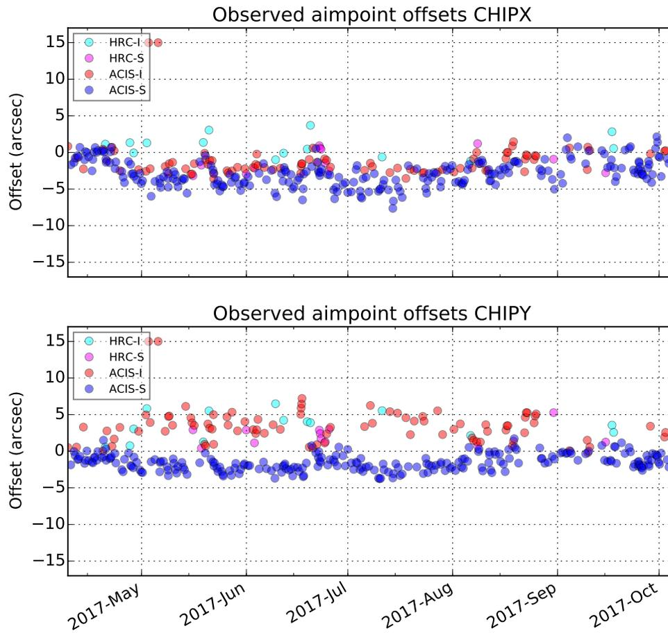
Figure 5.5: Difference between observed and planned aimpoint in CHIPX and CHIPY directions for recent observations with planned aimpoints within 100 arcsec of the nominal aimpoint.
