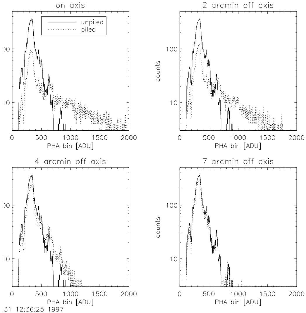
Figure 6.23: *MARX* simulations of the effect of pile-up on the shape of the spectrum. The true (solid line) and the detected (dotted line) spectra are shown for four different viewing angles. The corresponding “pile-up fractions” – see Section 6.16.2 – are 46%, 40%, 15%, and 2% as the image is moved progressively further off-axis.
