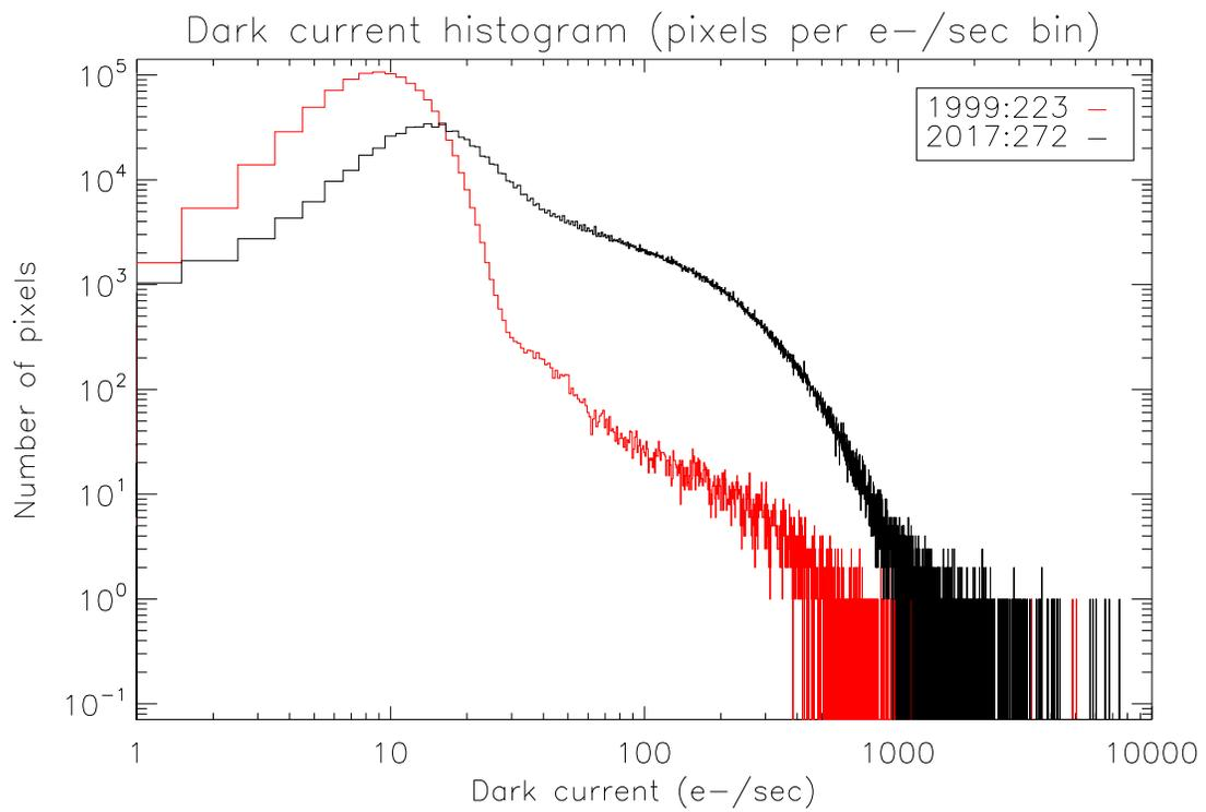
Figure 5.8: Differential histogram of dark current distribution for the ACA CCD in 1999-Aug and 2017-Sep
