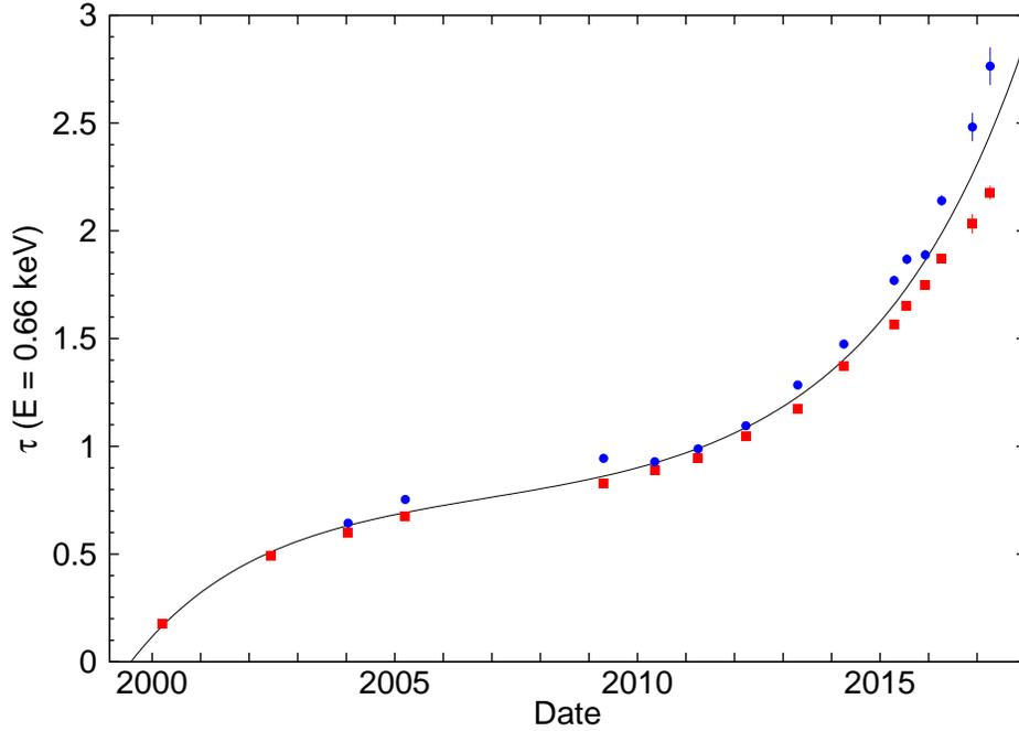
Figure 6.7: Optical depth of the contaminant measured at 0.66 keV from observations of the galaxy cluster Abell 1795. Light gray (red) squares denote observations with the target on ACIS-S and dark gray (blue) disks denote observations with the target on ACIS-I. The solid curve shows the best-fit relation to the data.
