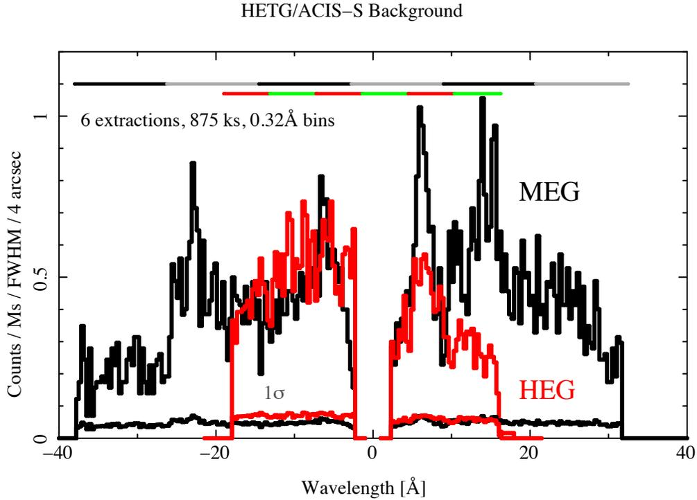
Figure 8.25: The first orders’ HETGS background count rate spectra, scaled to the spectral resolution along the dispersion axis and for the default cross-dispersion extraction width. The  $1\sigma$  uncertainties due to counting statistics are shown at the bottom. The approximate locations of each CCD, from S0 at the left to S5 at the right, are shown by the alternating color bars for the MEG (upper bar) and HEG (lower bar). This figure is adapted from a memo by Huenemoerder (2017).
