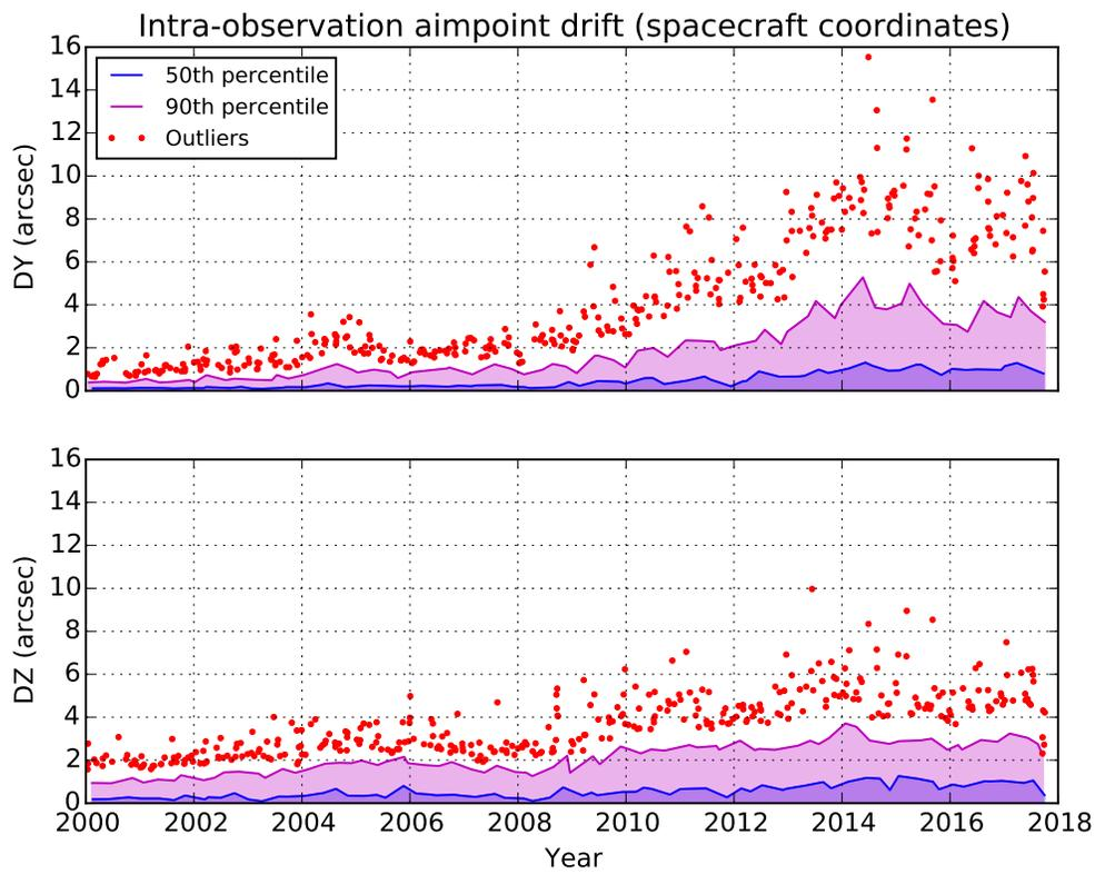
Figure 5.6: Peak to peak aimpoint drift within individual science observations. This figure shows that total intra-observation drift ( $DY+DZ$ ) up to  $6''$  during observations is possible and, in rare cases, drift over  $15''$  can occur.
