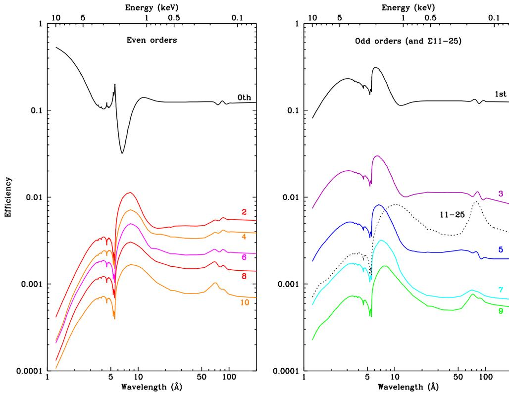
Figure 9.13: LETG grating efficiency. Combined positive and negative order efficiency is plotted versus wavelength and energy. For clarity, even and odd orders are plotted separately; the sum of orders 11–25 is also shown. Plotted values include all support structure diffraction. Net efficiency when using a spectral extraction region (see Figures 9.14 and 9.15) is 10–15% lower. Features near 6 and 80 Å are due to the partial transparency of the gold grating material at these wavelengths.
