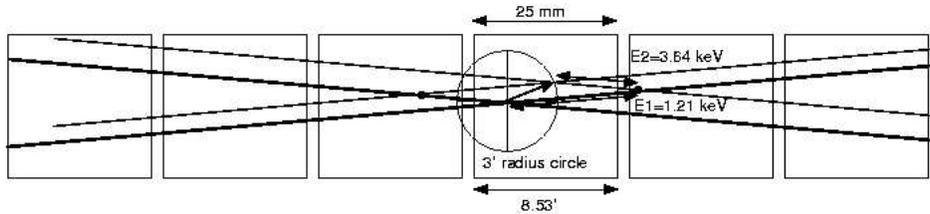
Figure 8.26: An idealized sketch of a ‘collision’ between two sources separated by 3 arcmin. At the ‘collision’ point, third-order photons from the on-axis source will have an energy  $3 \times 1.21 = 3.63$  keV and ACIS can not distinguish these from the second source’s first order photons, at 3.64 keV.
