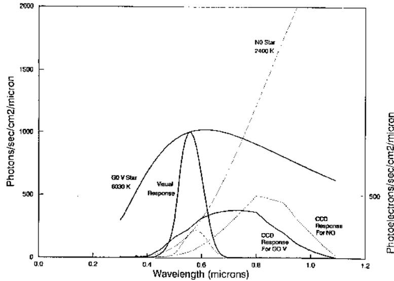
Figure 5.2: Spectral response of the ACA CCD. The same signal-to-noise is achieved for a  $V=11.7$  magnitude N0 star as for a  $V=10$  magnitude G0V star. Also shown are the spectra and the standard visual response for the two stars.
