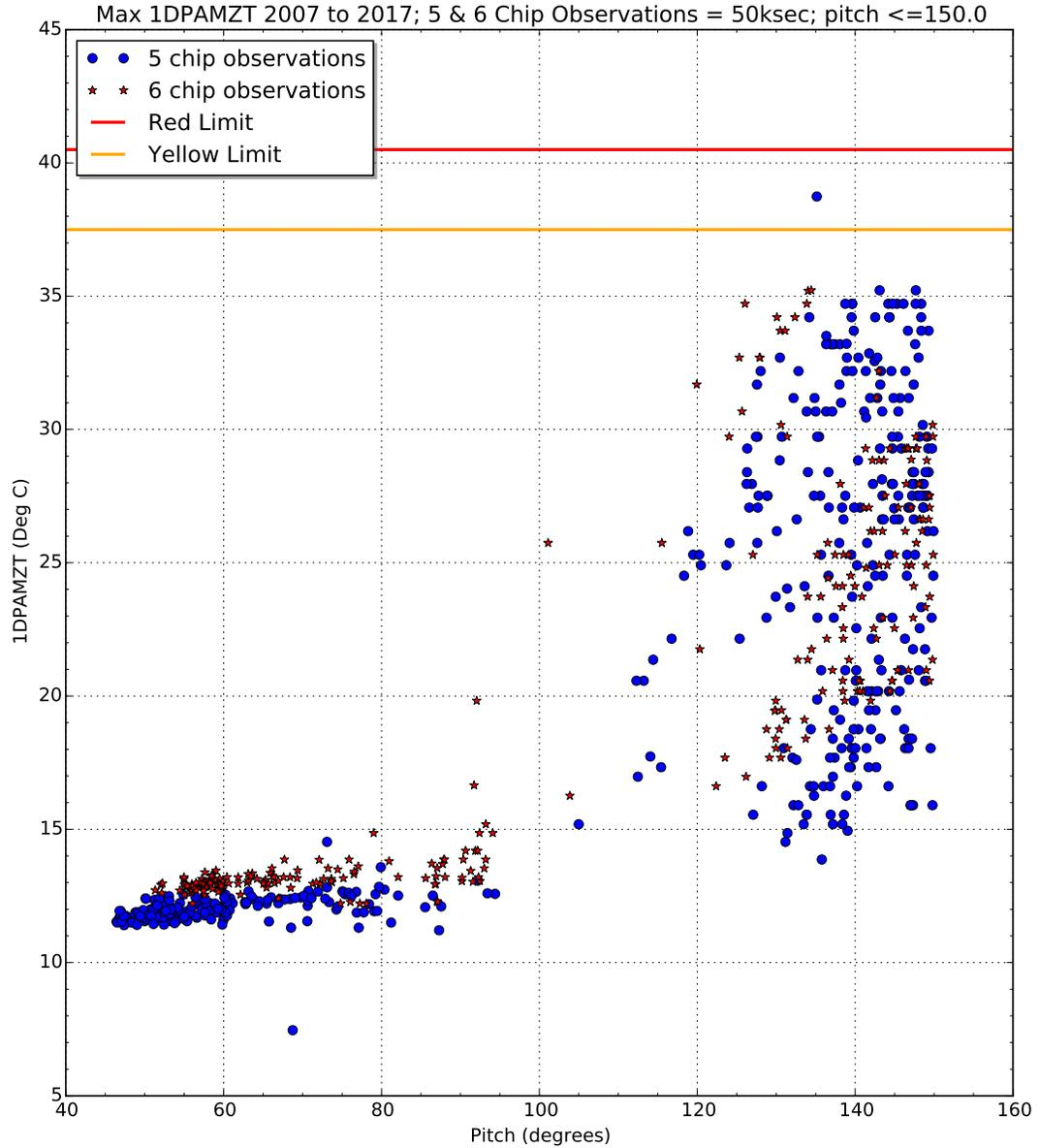
Figure 6.34: DPA temperature as a function of pitch angle for 5 and 6 CCD configurations. This figure shows the variation of DPA temperature with pitch angle. 6-CCD observations are indicated by small (red) stars, and 5-CCD observations are indicated by larger (blue) circles.
