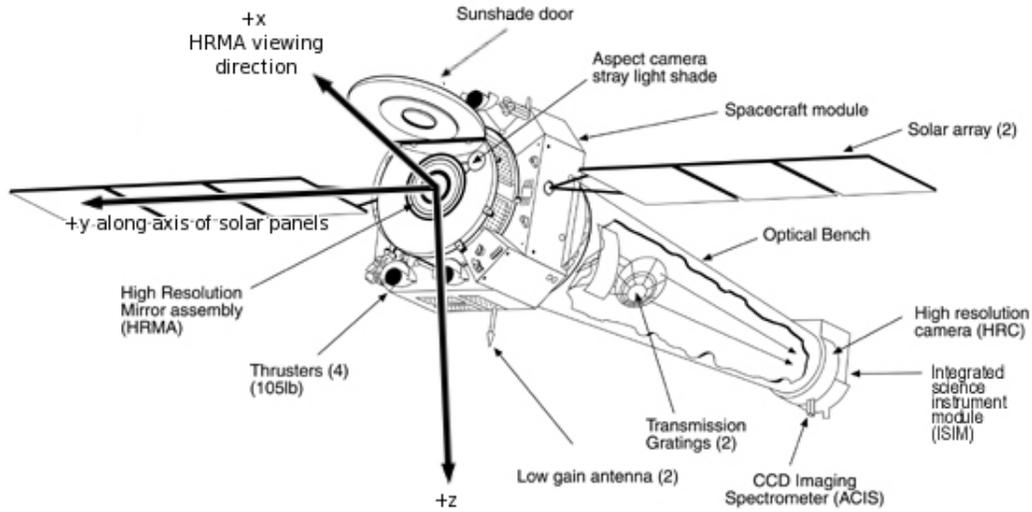
Figure 1.1: The *Chandra* Observatory with certain subsystems labeled.
