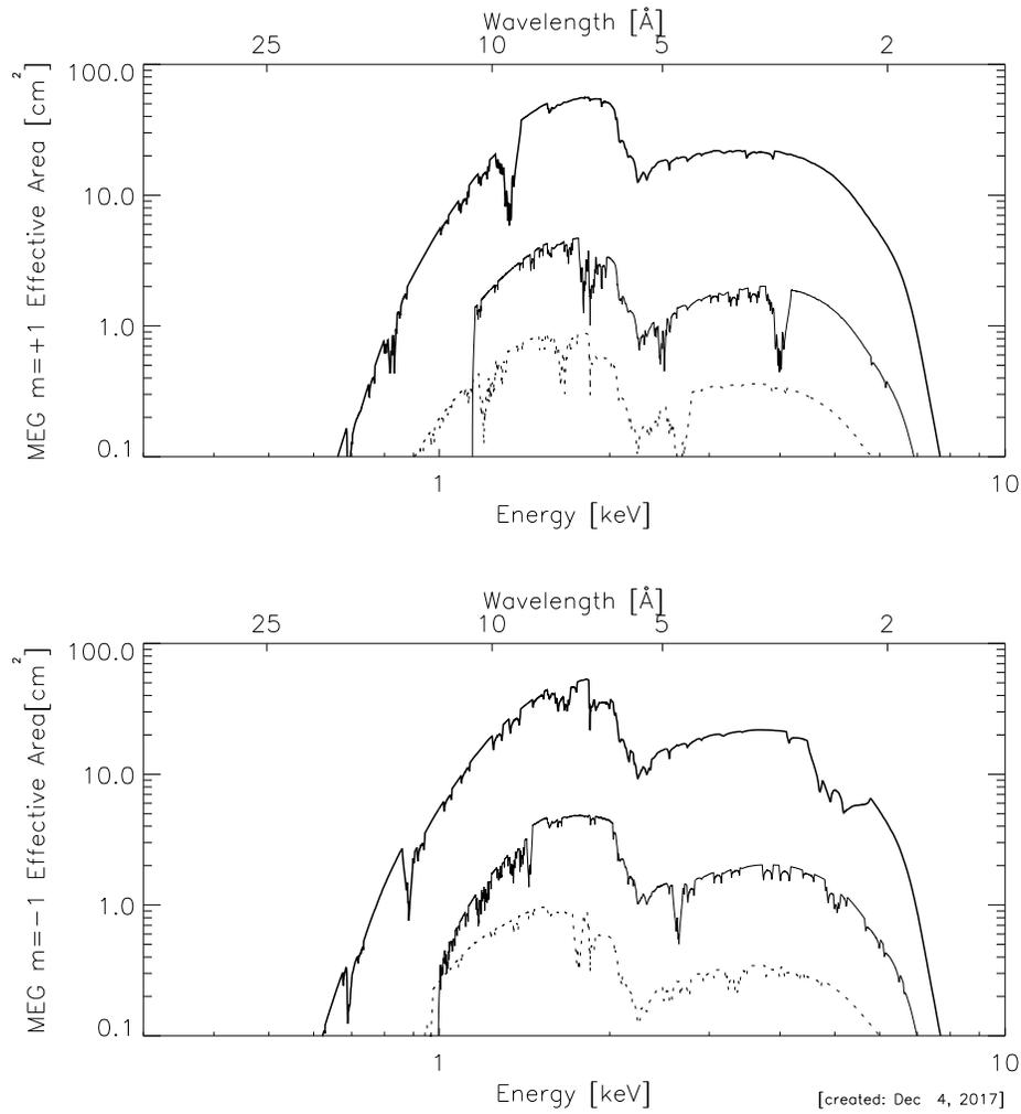
Figure 8.9: The HETGS MEG effective area, integrated over the PSF is shown with energy and wavelength scales. The  $m = +1, +2, +3$  orders (falling on ACIS chips S5, S4, S3; left to right) are displayed in the top panel and the  $m = -1, -2, -3$  orders (falling on ACIS chips S0, S1, S2; left to right) are in the bottom panel. The thick solid lines are first order; the thin solid line is third order; and the dotted line is second order.
