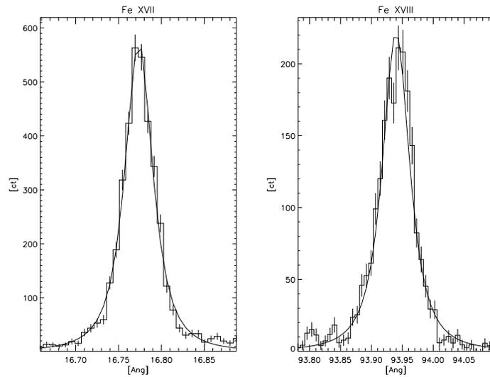
Figure 9.9: LETGS line response function as illustrated by two bright Fe lines (Fe XVII at  $\sim 17 \text{ \AA}$  and Fe XVIII at  $\sim 94 \text{ \AA}$ ) using in-flight calibration observations of Capella. The solid curves are best-fit Moffat functions with  $\beta = 2.5$ .
