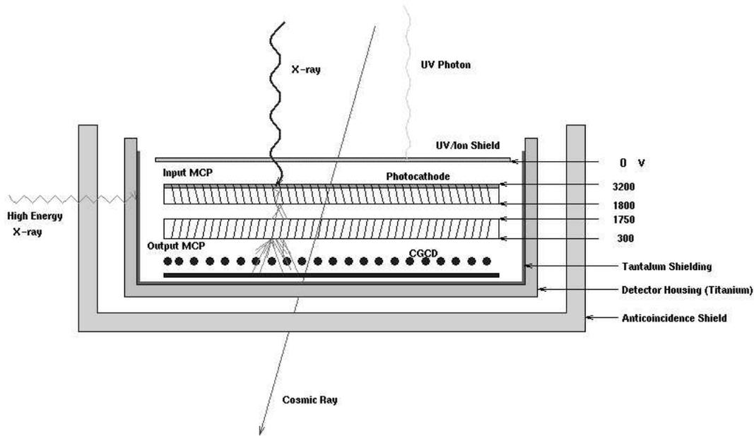
Figure 7.3: A schematic of the HRC Microchannel-Plate detector.
