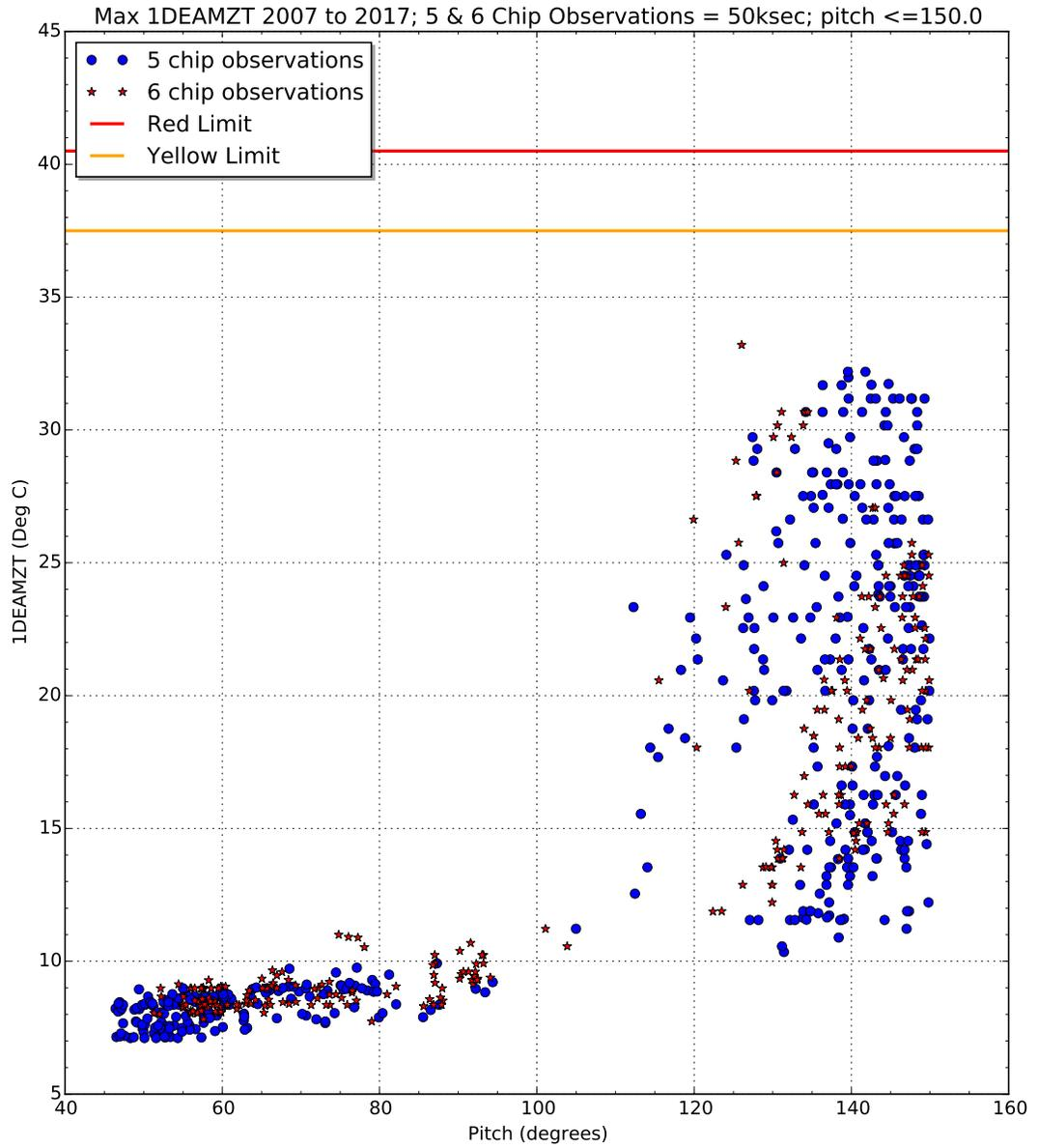
Figure 6.35: DEA temperature versus pitch angle for 5 and 6 CCD observations. This figure shows the variation of DEA temperature with pitch angle. 6-CCD observations are indicated by small (red) stars, and 5-CCD observations are indicated by larger (blue) circles.
