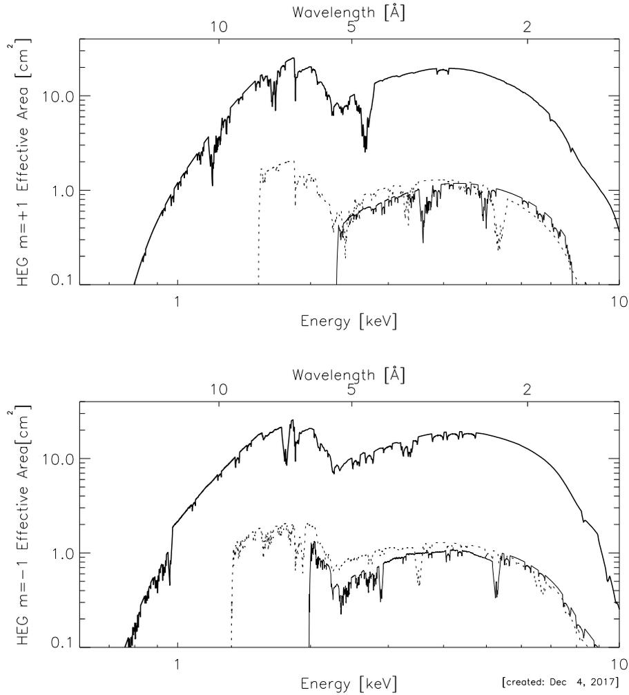
Figure 8.7: The HETGS HEG effective area, integrated over the PSF, is shown with energy and wavelength scales. The  $m = +1, +2, +3$  orders (falling on ACIS chips S5, S4, S3; left to right) are displayed in the top panel and the  $m = -1, -2, -3$  orders (falling on ACIS chips S0, S1, S2; left to right) are in the bottom panel. The thick solid lines are first order; the thin solid line is third order; and the dotted line is second order.
