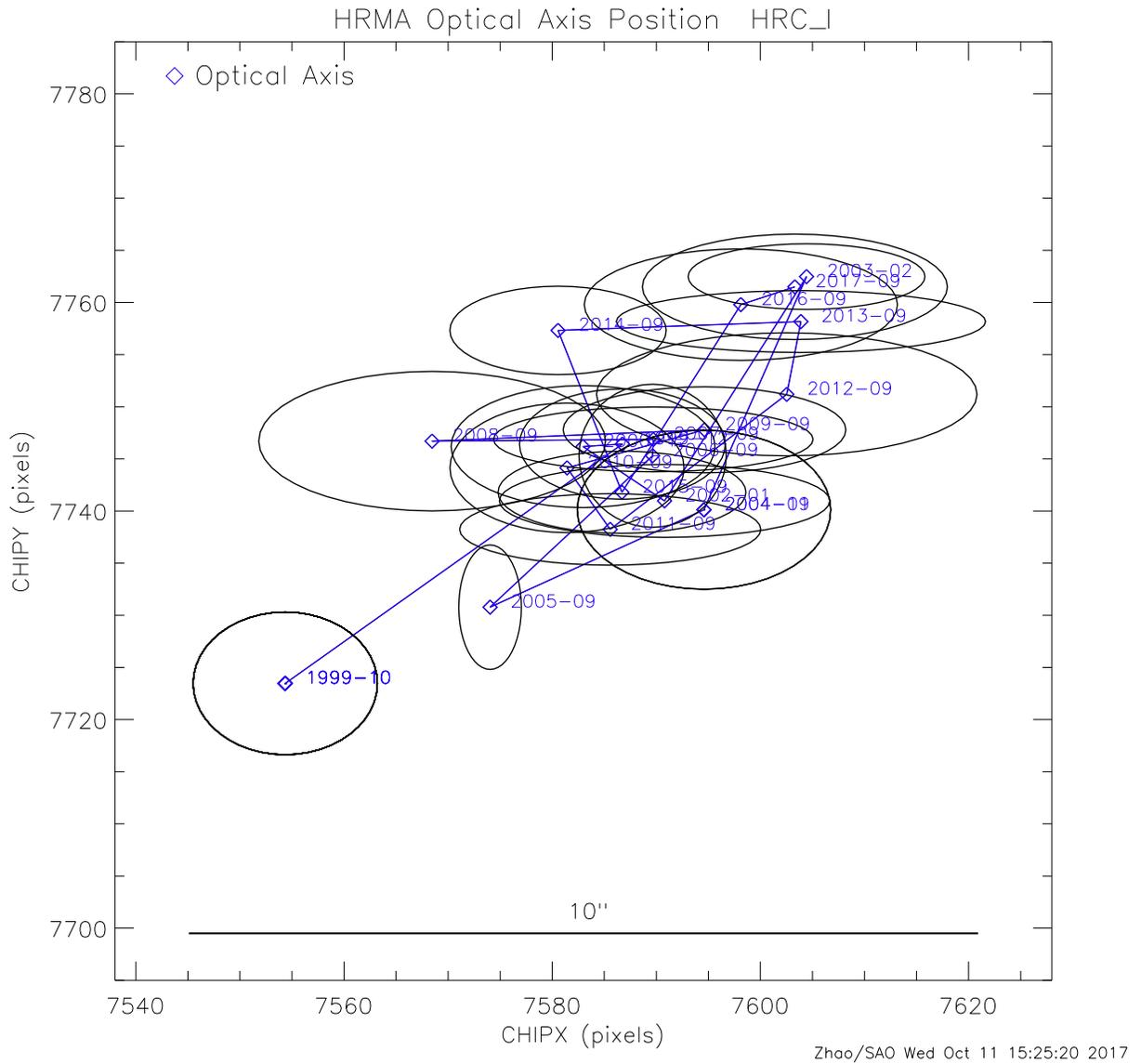
Figure 4.25: *Chandra* optical axis positions on HRC-I since launch. Each position is labeled by the year-month. The ellipse around each position is the  $1 - \sigma$  measurement error ellipse for that given year. The drift of optical axis position is consistent with the measurement errors. The optical axis position is very stable and well within a  $10''$  region. Since year 2000, the optical axis drift was well within a  $6''$  region.
