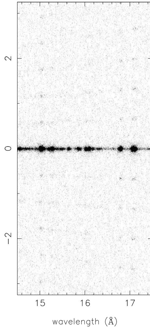
Figure 9.24: Detail of Figure 9.23, showing the LETG/HRC-S image of bright lines in Capella. Vertical and horizontal scales are identical. The Fe XVII lines at  $\sim 15$  and  $17$  Å are the brightest in the LETG Capella spectrum. Faint features above and below the primary spectrum are due to fine support structure diffraction.
