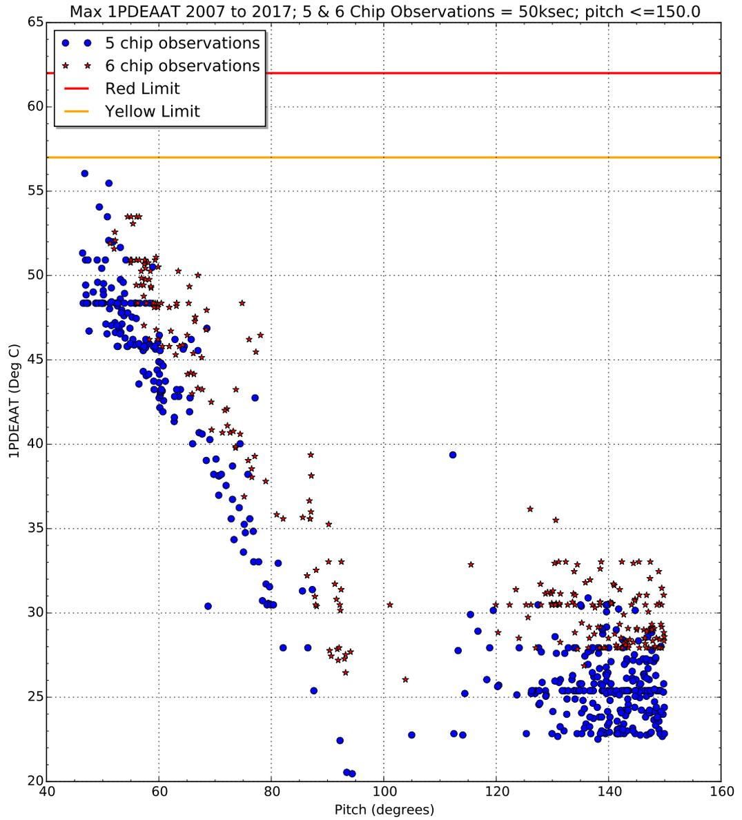
Figure 6.33: ACIS PSMC temperature as a function of spacecraft pitch angle 6-CCD observations are indicated by small (red) stars, and 5-CCD observations are indicated by larger (blue) circles.
