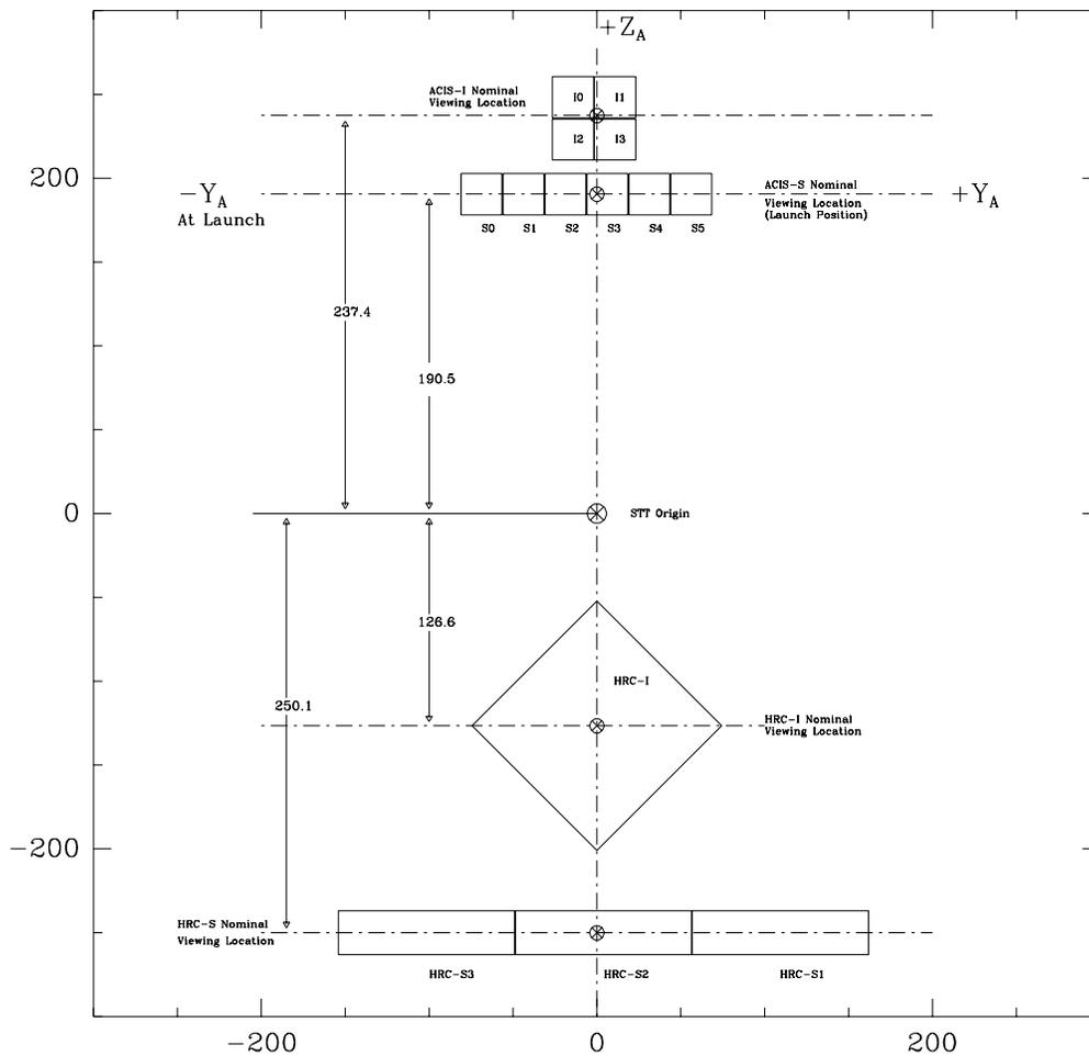
Figure 4.24: Layout of *Chandra* Detectors: The schematic of the SIM plane shows the *Chandra* focal plane instrument to scale (mm). SIM  $+Y$  is along the x-axis; SIM  $+Z$  is along the y-axis.  $\otimes$  on each detector marks the aimpoint position with nominal SIM-Z position and zero pointing offset.
