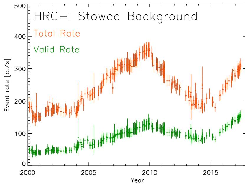
Figure 7.20: The change in HRC-I stowed background rate with time. The total rate (red points and error bars, upper set) and the valid rate (black points and error bars, lower set) are shown. The HRC-S data are similar.
