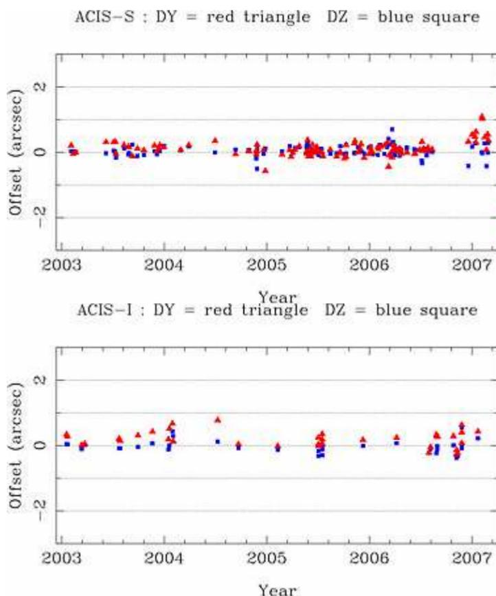
Based on this evidence that the ACA CCD cooling operation can affect the aspect fiducial transfer system alignment, the aspect offsets since Jan-2003 have been analyzed to determine optimal alignment values for each of the three operational ACA CCD temperature values (-10 C, -15 C, and -19 C). The new CALALIGN files are version N0006.
