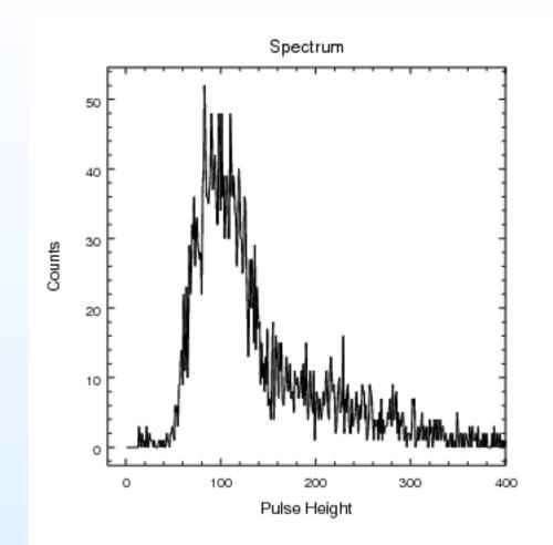
**Figure 1.** A typical Chandra X-ray spectrum, from data observed with the ACIS detector. ACIS consists of a number of CCD chips that can record not only a photon's position on the detector, but also its energy and time of arrival. When ACIS data are binned by energy, an X-ray spectrum for the observation is created. However, the observed X-ray spectrum is not flux vs. energy (or wavelength), but rather number of detected counts vs. pulse height amplitude for detector channels.
