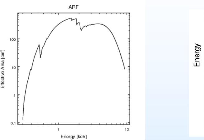
Figure 2. Effective area curve for chip 1 of the Chandra ACIS detector. The effective area varies as a function of energy, quite significantly. This variation must be included in a model fitted to a Chandra observation.
