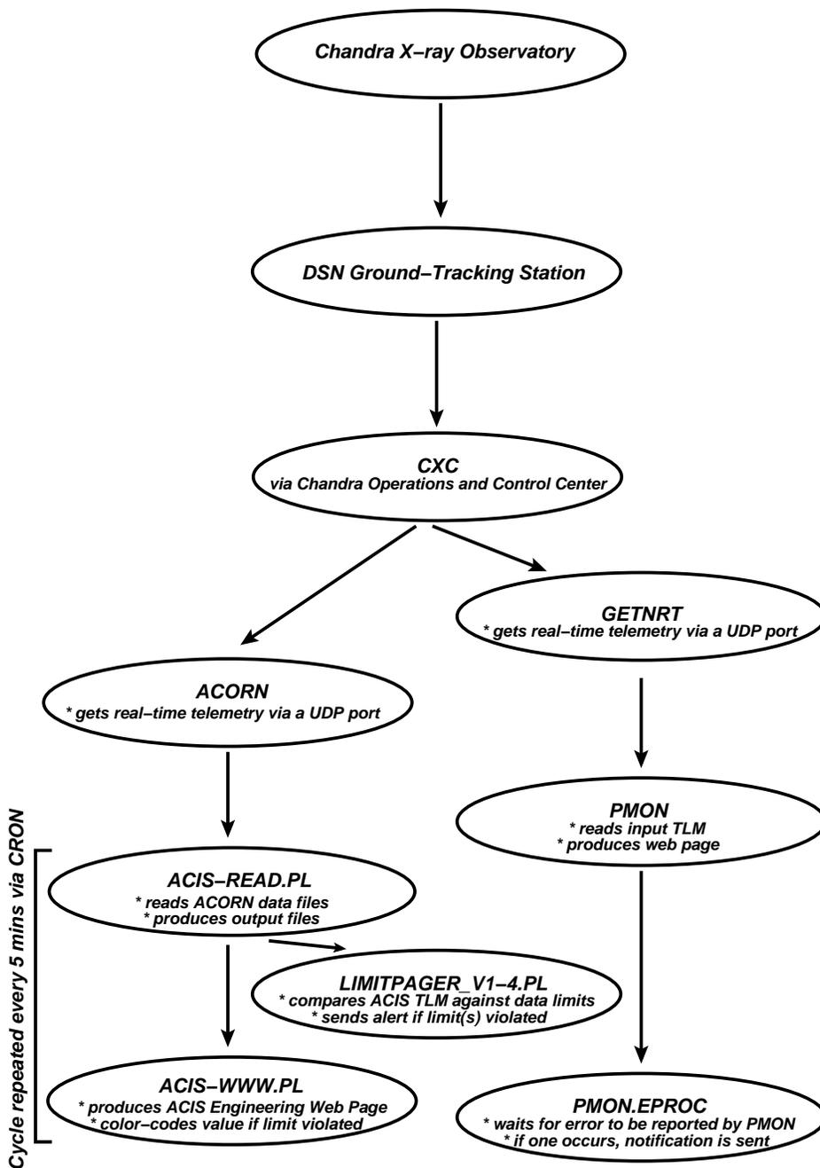
**Figure 1.** Real-time Data Flow: The pathway by which real-time telemetry from the spacecraft results in ACIS monitoring web pages.
