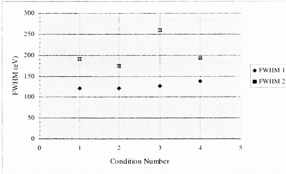
Figure 6. The change in FWHM from fitting the  $\text{MnK}\alpha$  line with two Gaussians and a constant.
