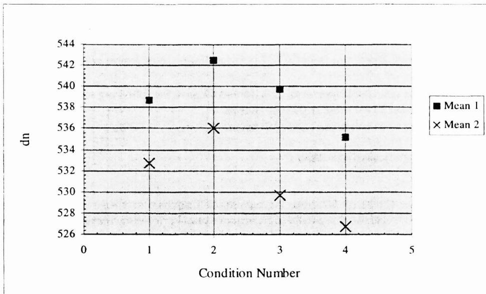
Figure 7. The change in gain from fitting the  $\text{MnK}\alpha$  line with two Gaussians and a constant.
