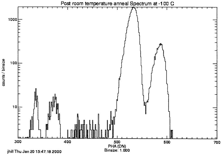
Figure 5. Spectrum from CCID7 post-irradiation, post anneal at -100 C.
