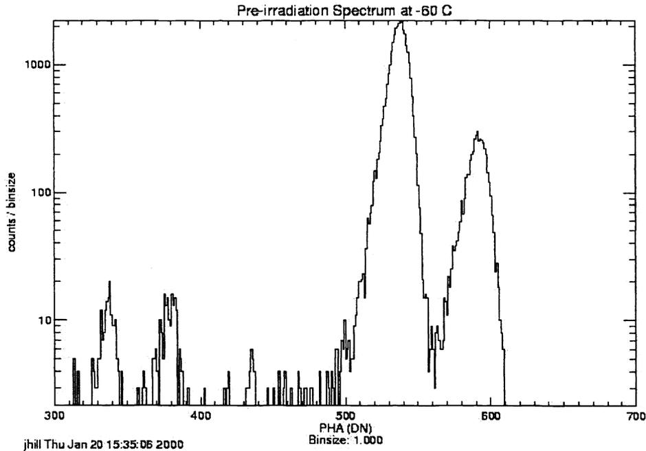
Figure 1. Mn spectrum from CCID7, pre-irradiation at -60C
