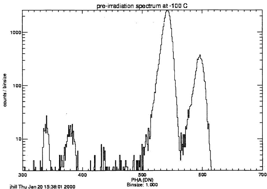
Figure 2. Spectrum from CCID7, pre-irradiation, at -100 C.
