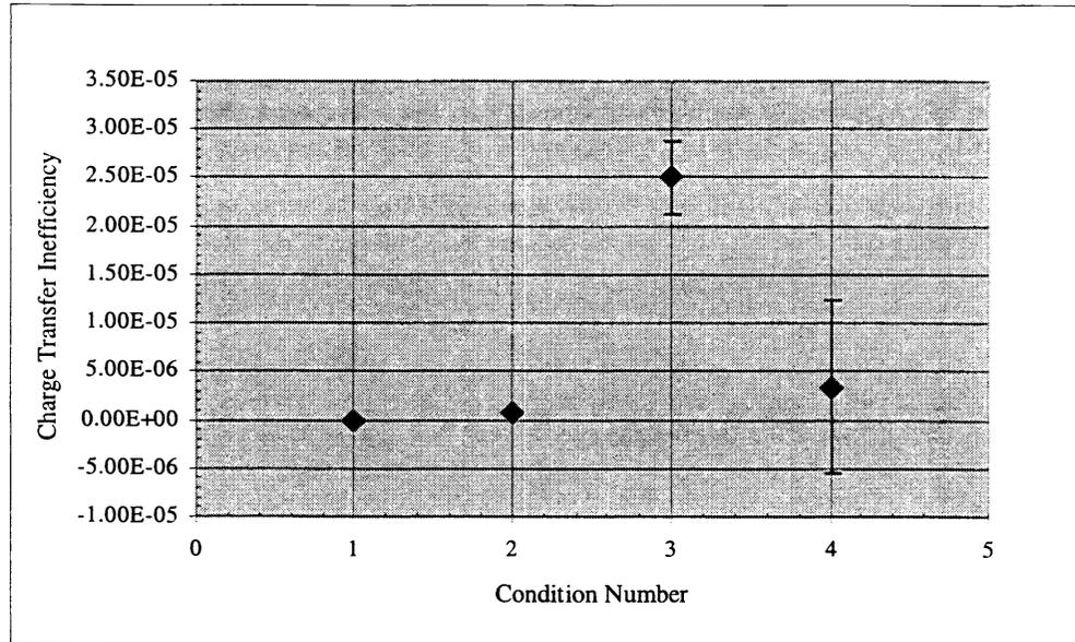
Figure 8. Charge transfer efficiency as a function of CCD condition.
