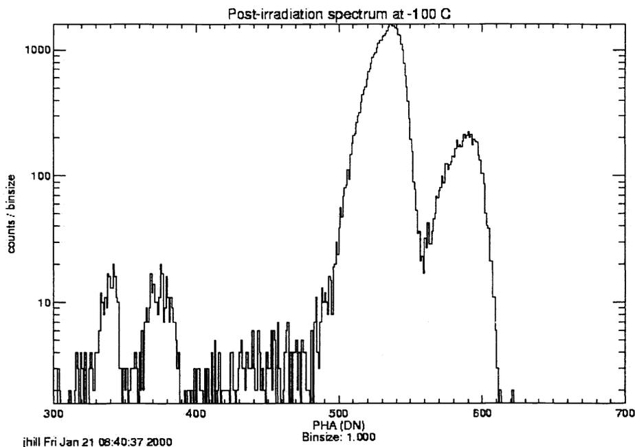
Figure 4. Spectrum from CCID7 post-irradiation.
