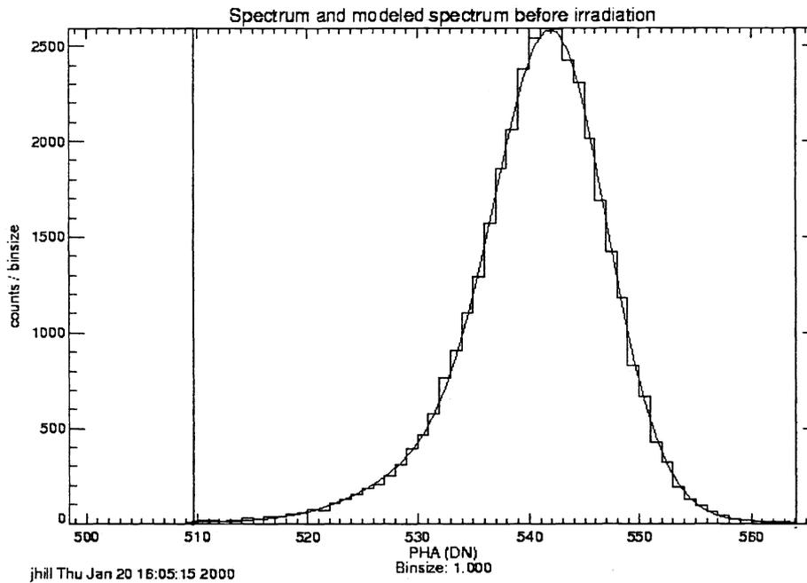
Figure 3. MnK $\alpha$  spectral fit from CCID7 pre-irradiation.
