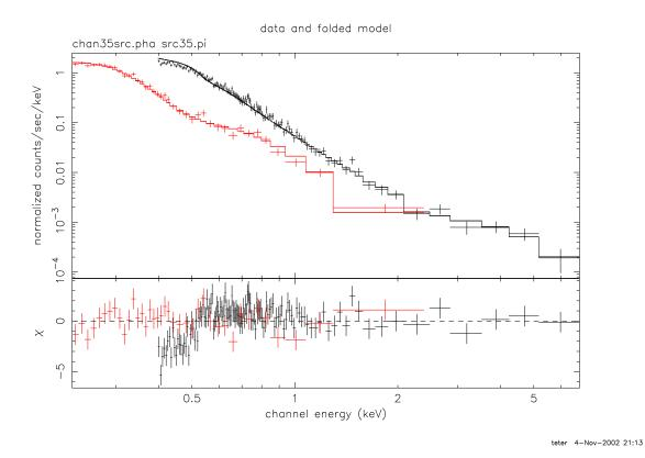
Pulsar 1055 fit to PSPC and ACIS above 0.9 keV without the ACISABS contamination model. Shows deviation of ACIS spectrum.
