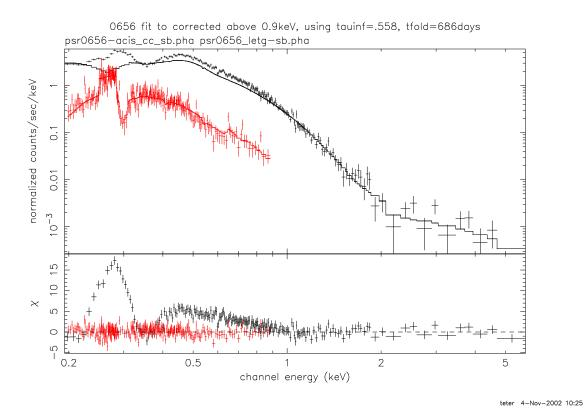
No Fitting. Adjusted contamination layer model to minimum values for the parameters in equation 1:  $\tau_{\infty}=0.558$ ,  $t_{fold}=686$  days. The overcorrection is improved slightly.
