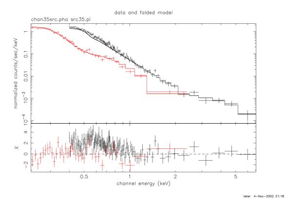
Pulsar 1055 fit to PSPC and ACIS above 0.9 keV with the default ACISABS contamination model. Clear overcorrection seen.
