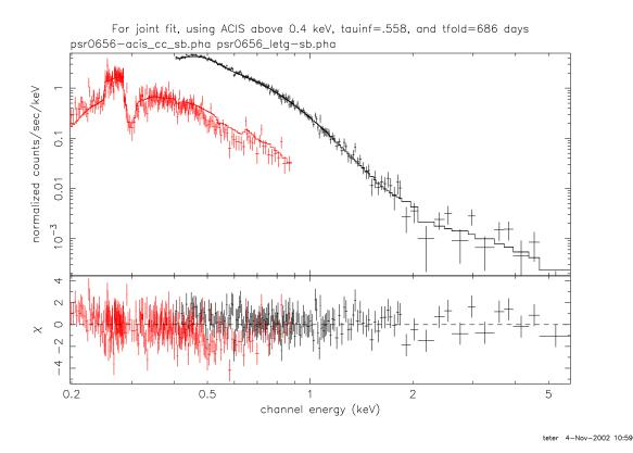
Pulsar 0656 fit to LETGS below 1.0 keV and ACIS above 0.4 keV using the contamination model. Adjusted contamination layer model to minimize correction.  $\tau_{\infty} = 0.558$ ,  $t_{fold} = 686$  days. The overcorrection seems to disappear, but it can be seen in the residuals for the LETGS.
