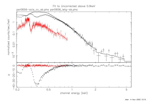
Pulsar B0656+14 fit to LETGS below 1.0 keV and ACIS above 0.9 keV. The ACIS residuals show the large deviation due to the contamination layer.
