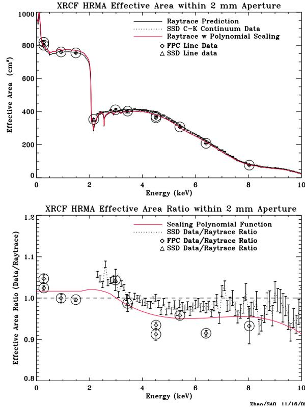
**Fig. 7.** SAOSAC raytrace code predictions for the HRMA effective area at XRCF along with ground-based measurements.
