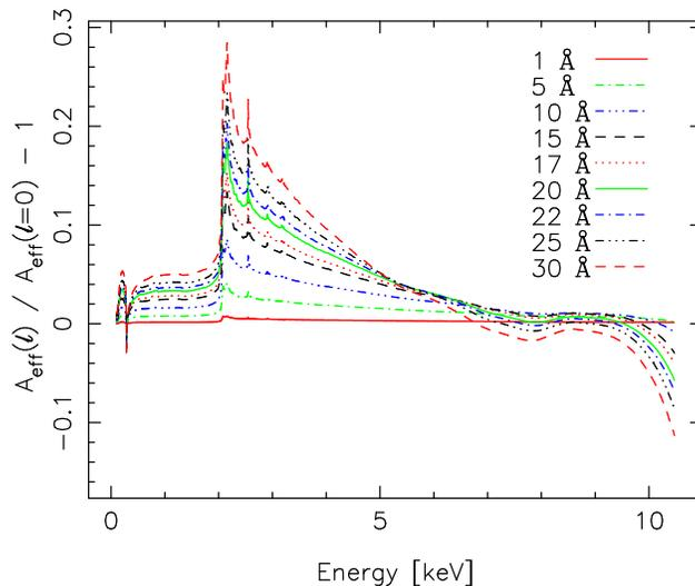
**Fig. 9.** The effects of an overlayer of hydrocarbon on the HRMA effective area.
