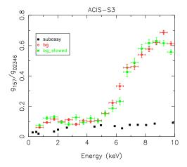
Figure A.1: Ratio of ASCA "bad" grades to ASCA "good" grades for ACIS-S3 sub-assembly data and ACIS-S3 on-orbit background data. The subassy data are from subassembly calibration test during ground testing. The bg and bg\_stowed datasets are level 1 background datasets. bg is blank sky background, and bg\_stowed is background taken when ACIS was out of the focal plane and not exposed to the sky. See text.
