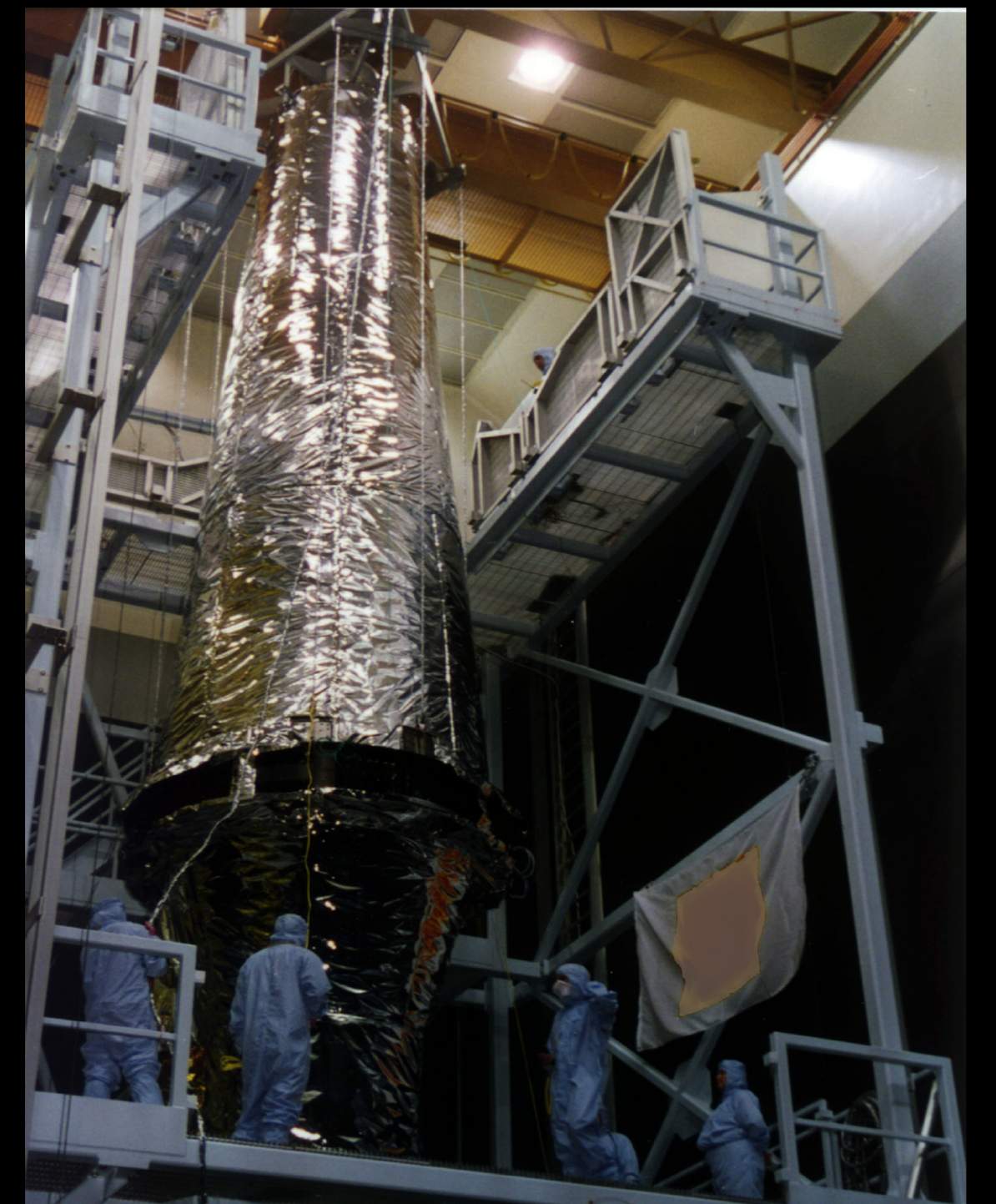
Optical Bench Assembly and High Resolution Mirror Assembly (HRMA) integration
