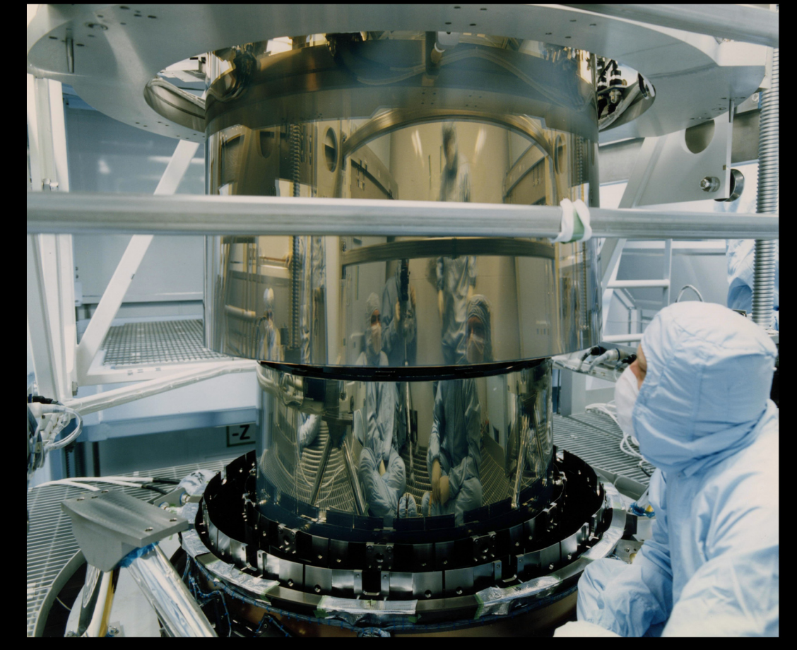
All H-mirrors installed. Note MAS interface points on the tops of the mirrors
