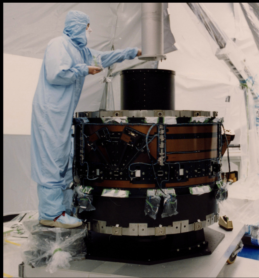
All P-mirrors installed. Note CAP Offloaders/Hardpoints
