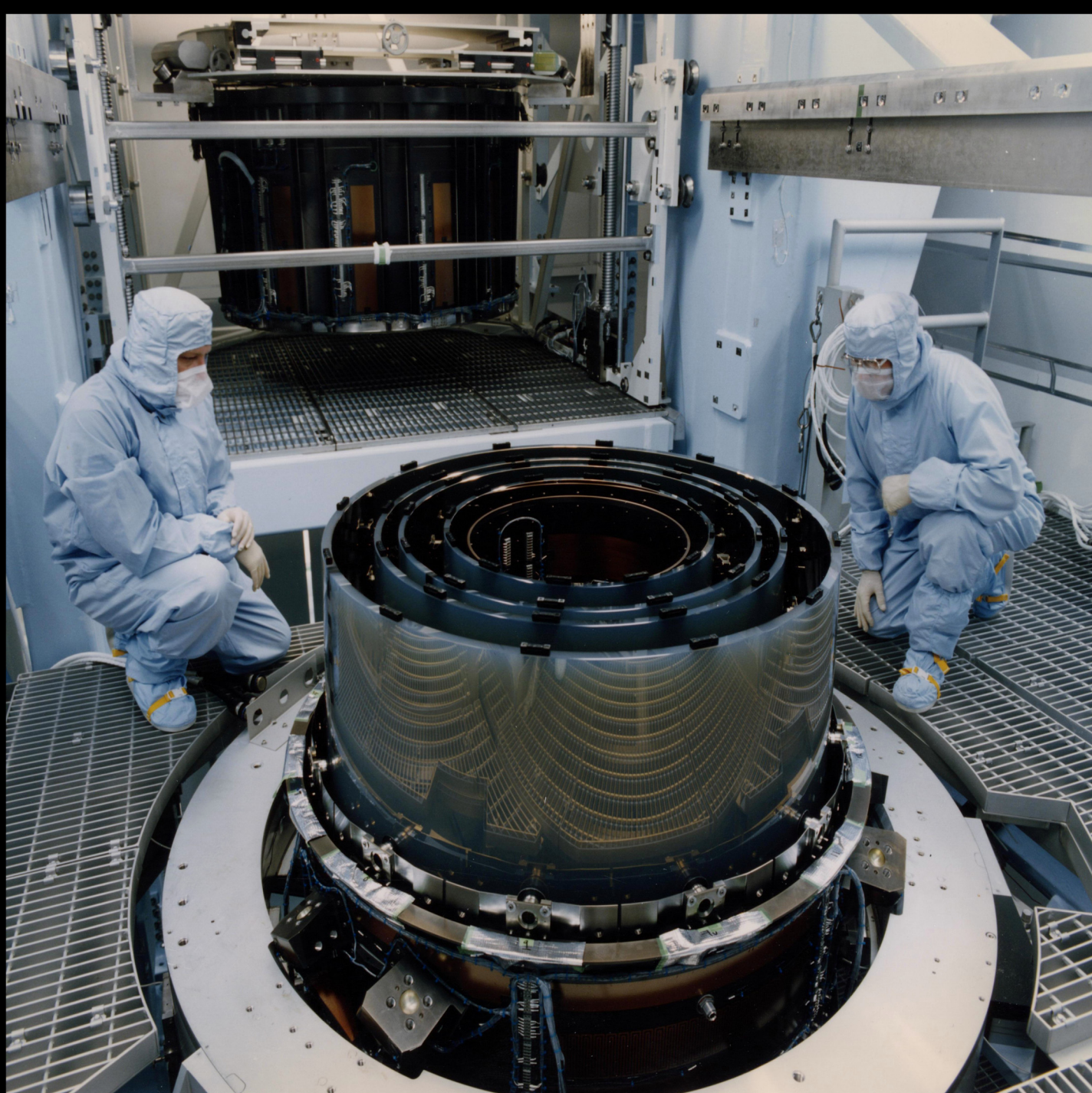
Final inspection of P-mirrors. Note Pre-Collimator in the background
