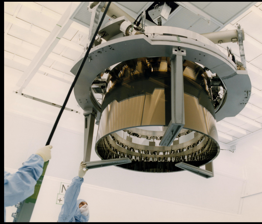
All P-mirrors installed. Note CAP Offloaders/Hardpoints
