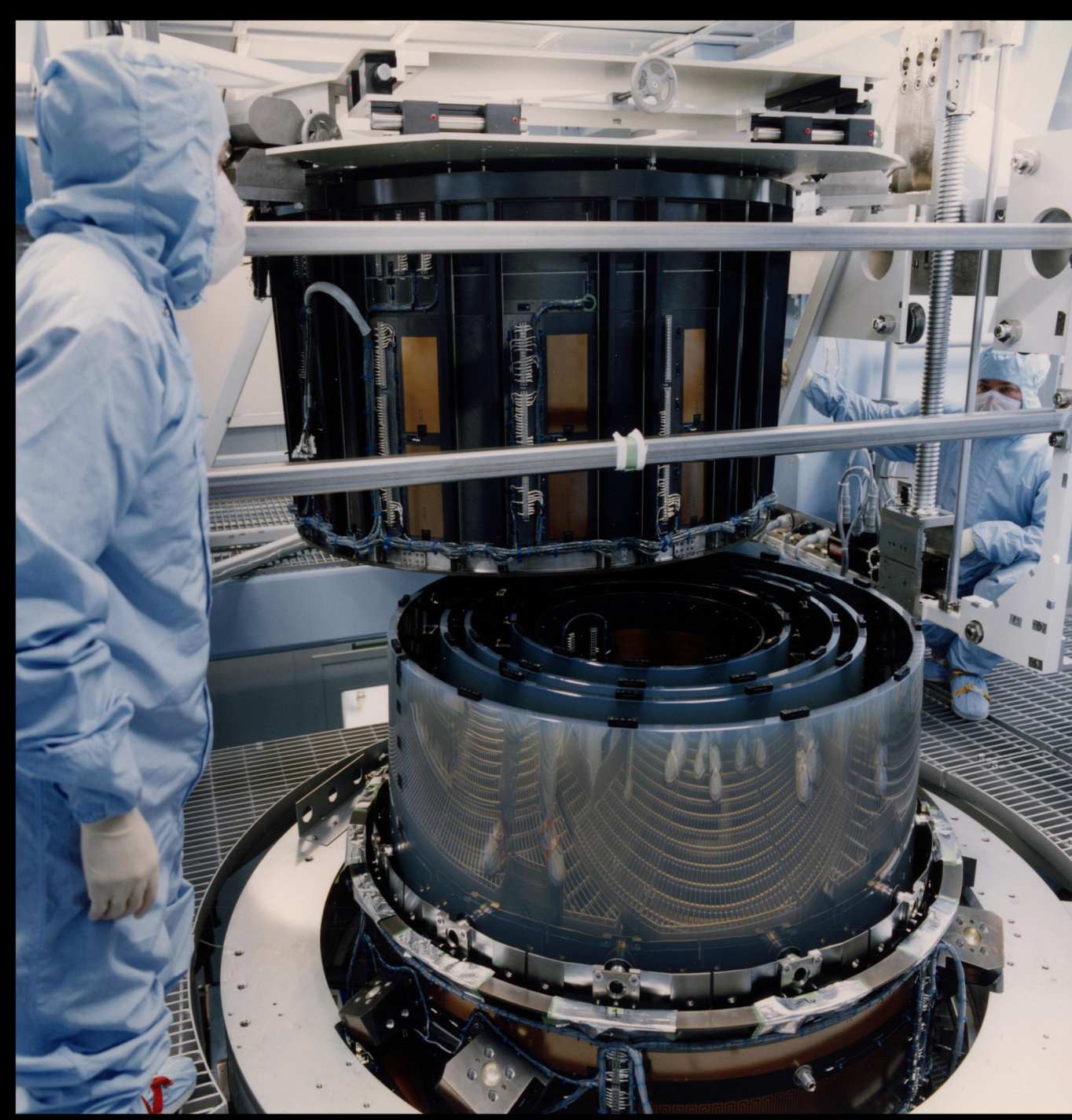
Post Collimator being integrated onto the HRMA structure
