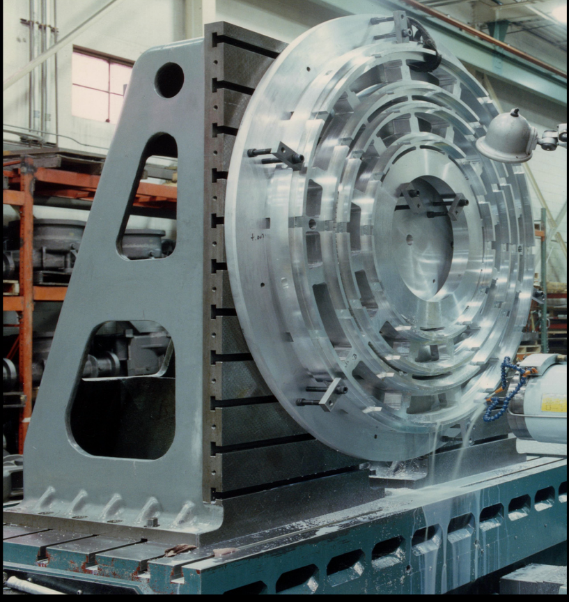
Center Aperture Plate during machining
