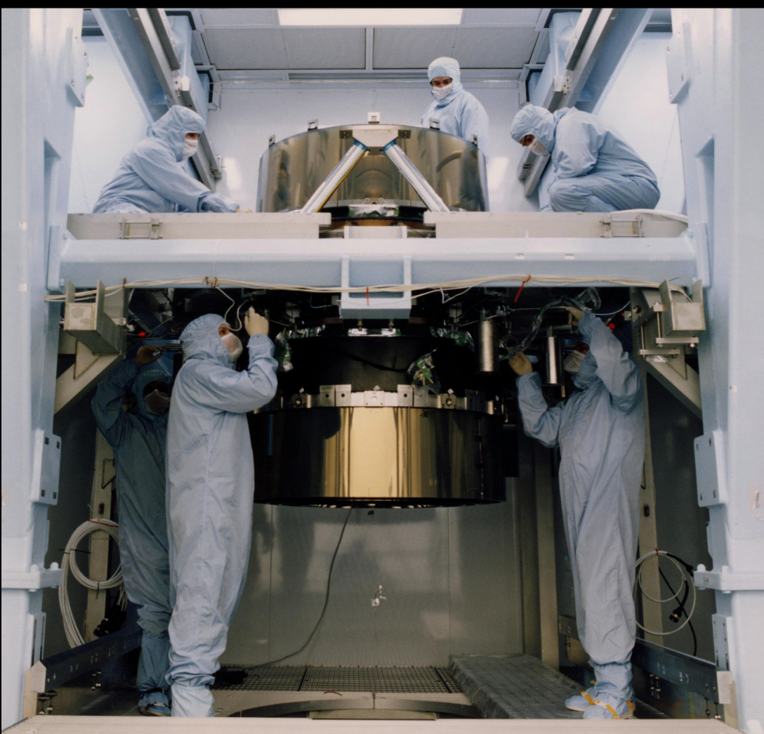
Final inspection of P-mirrors. Note Pre-Collimator in the background
